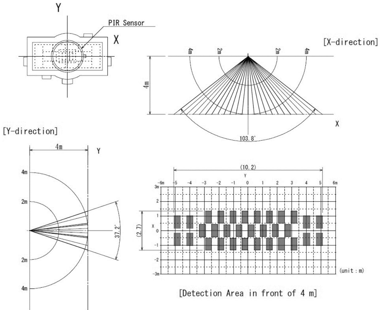
**Figure 3 – ZNCL11 Detection Area with Dual Element PIR**
