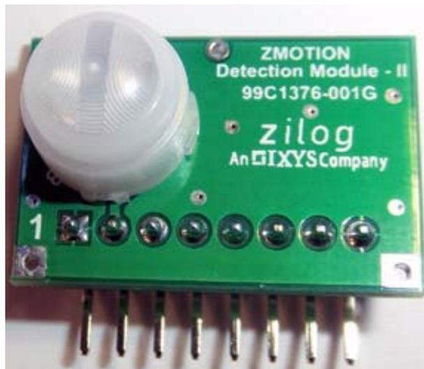
Figure 2. The ZMOTION Detection Module II, Right-Angle Version (ZEPIR0BAS02MODG)
