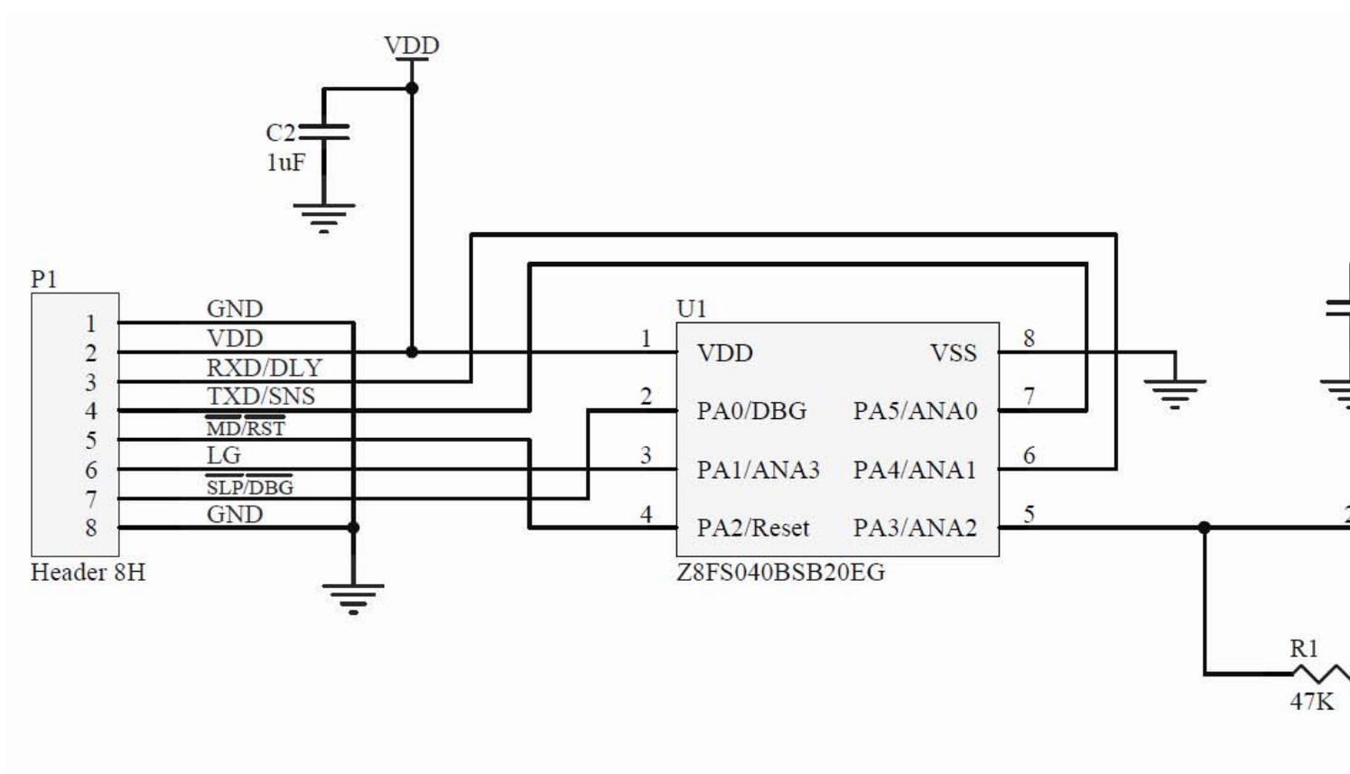
Figure 11. Schematic Diagram of ZMOTION Detection Module II
