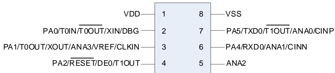
Figure 2. 8-Pin SOIC Package Diagram – Z8FS040xSB20EG
