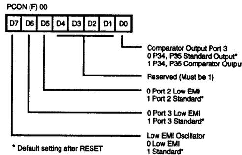
Figure 17. Port Configuration Register (PCON) (Write Only)
