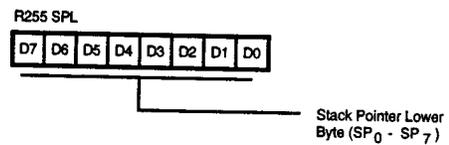
Figure 51. Stack Pointer (FF<sub>n</sub>: Read/Write)
