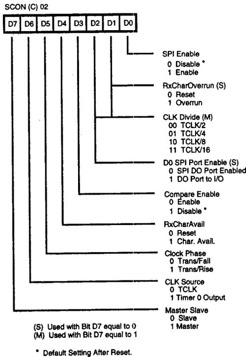
**Figure 13. SPI Control Register (SCON)
