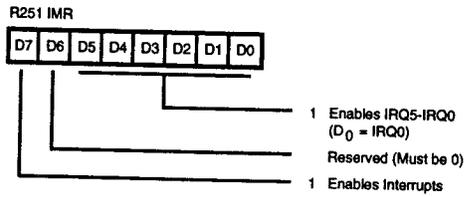
Figure 47. Interrupt Mask Register (FB<sub>n</sub>: Read/Write)
