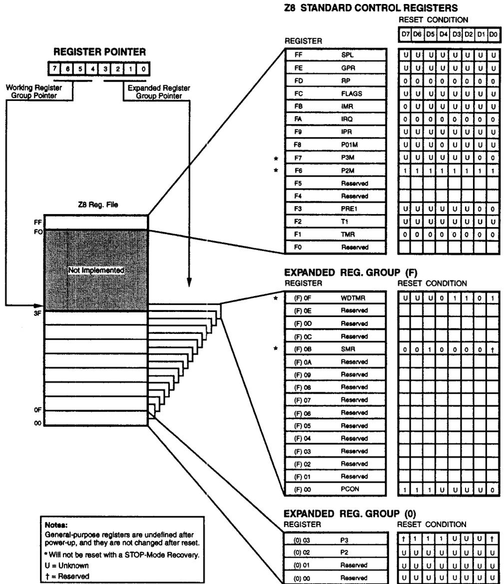
Figure 7a. Expanded Register File Architecture (Z86E03)
