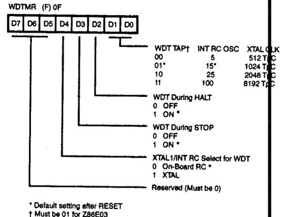
Figure 20. Watch-Dog Timer Mode Register (Write Only)
