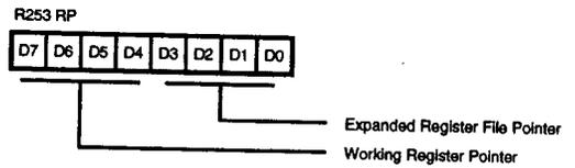
Figure 49. Register Pointer (FD<sub>n</sub>: Read/Write)
