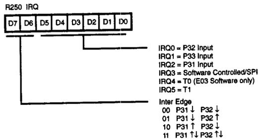
Figure 46. Interrupt Request Register
