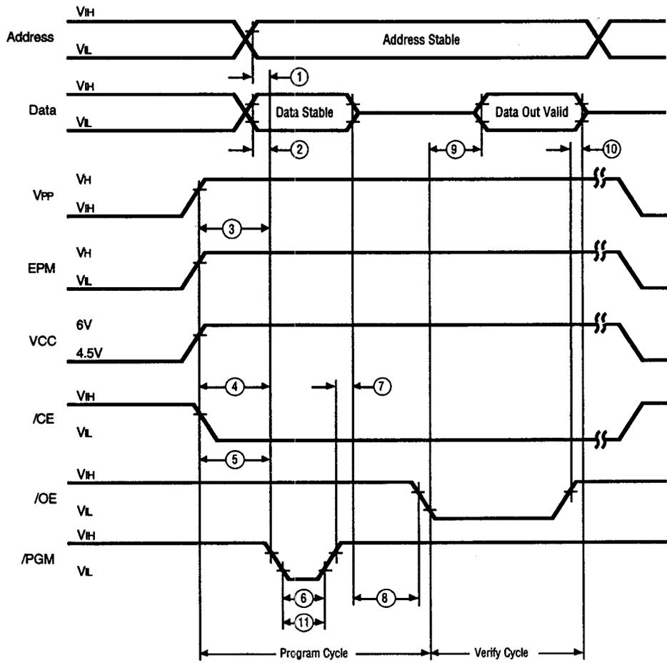
**Figure 25. Z86E03/E06 Programming Waveform (Program and Verify)**
