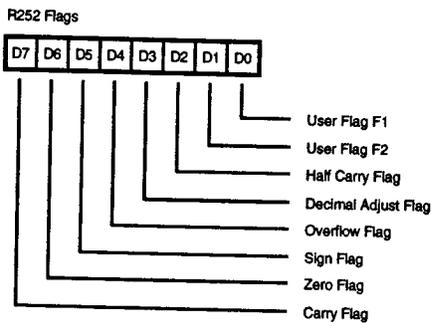
Figure 48. Flag Register (FC<sub>n</sub>: Read/Write)
