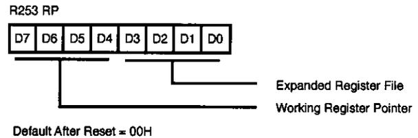
Figure 36. Register Pointer
