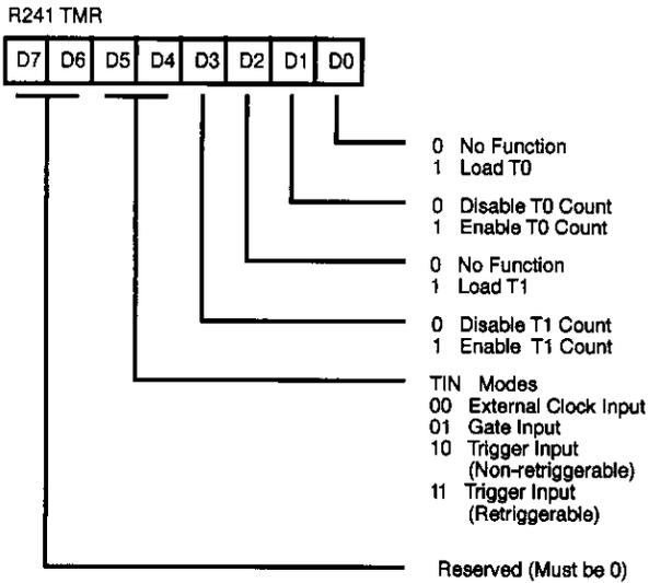
Figure 24. Timer Mode Register (F1<sub>H</sub>: Read/Write)
