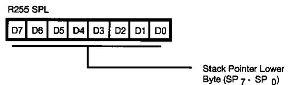
Figure 37. Stack Pointer
