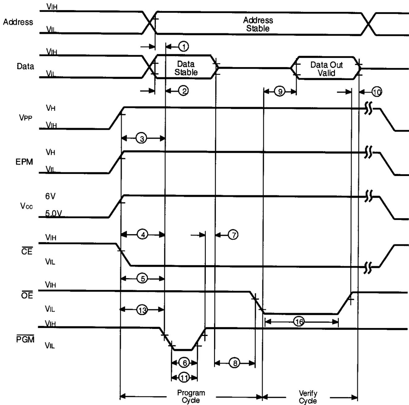
Figure 20. Z86E04/E08 Programming Waveform (Program and Verify)
