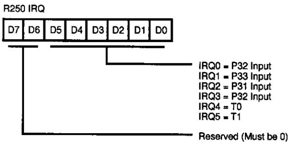
Figure 33. Interrupt Request Register
