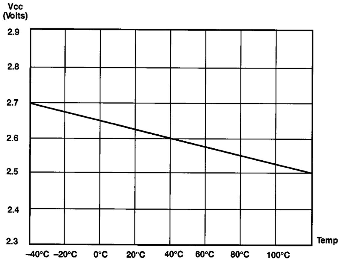
Figure 17. Typical Auto Reset Voltage (V<sub>LV</sub>) vs. Temperature
