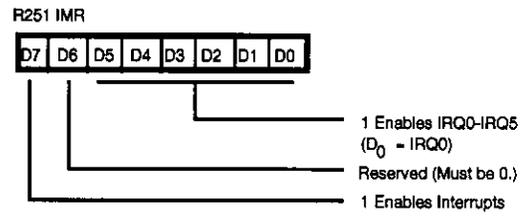
Figure 34. Interrupt Mask Register
