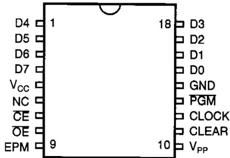
Figure 3. 18-Pin EPROM Mode Configuration
