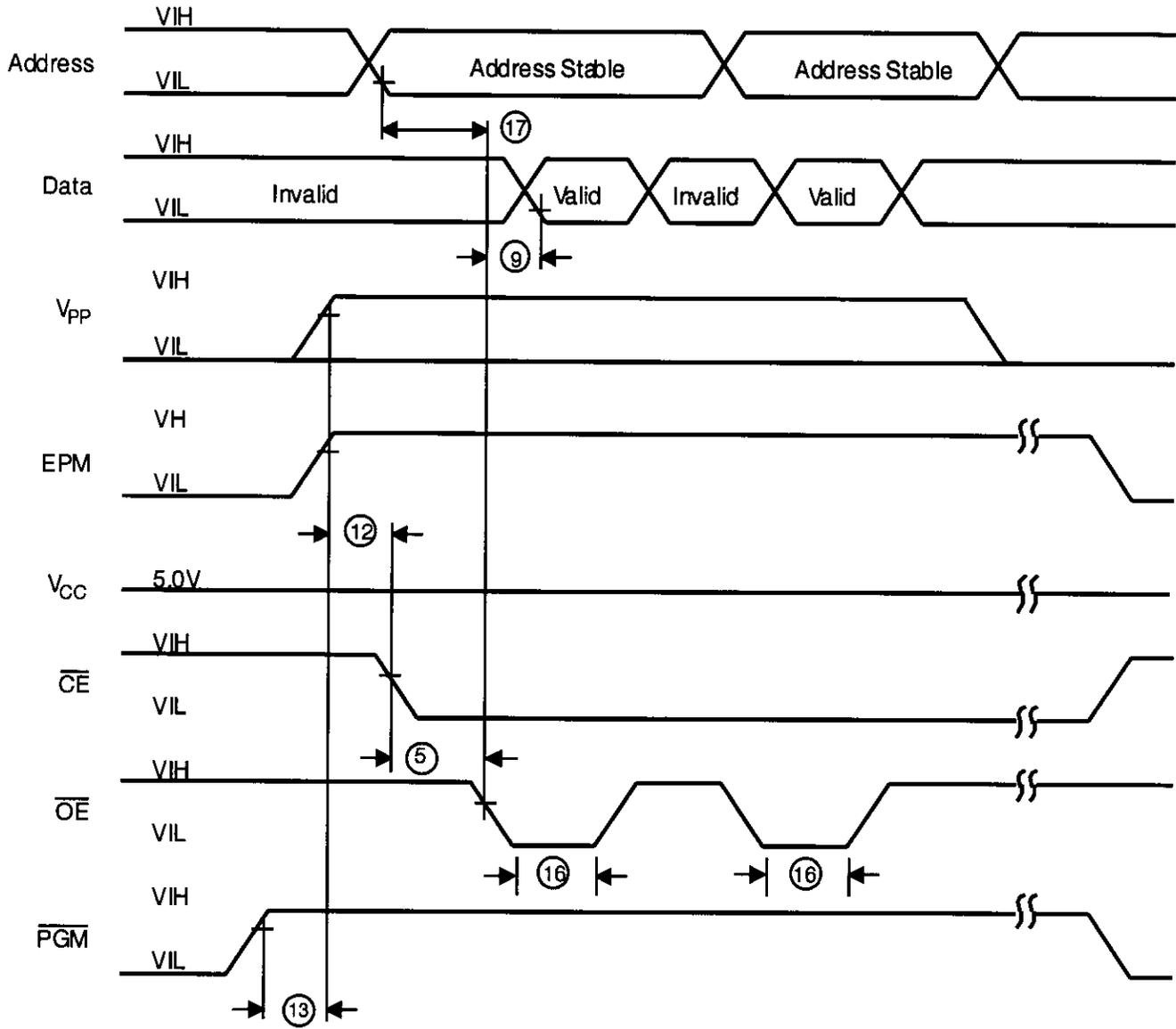
Figure 19. Z86E04/E08 Programming Waveform
