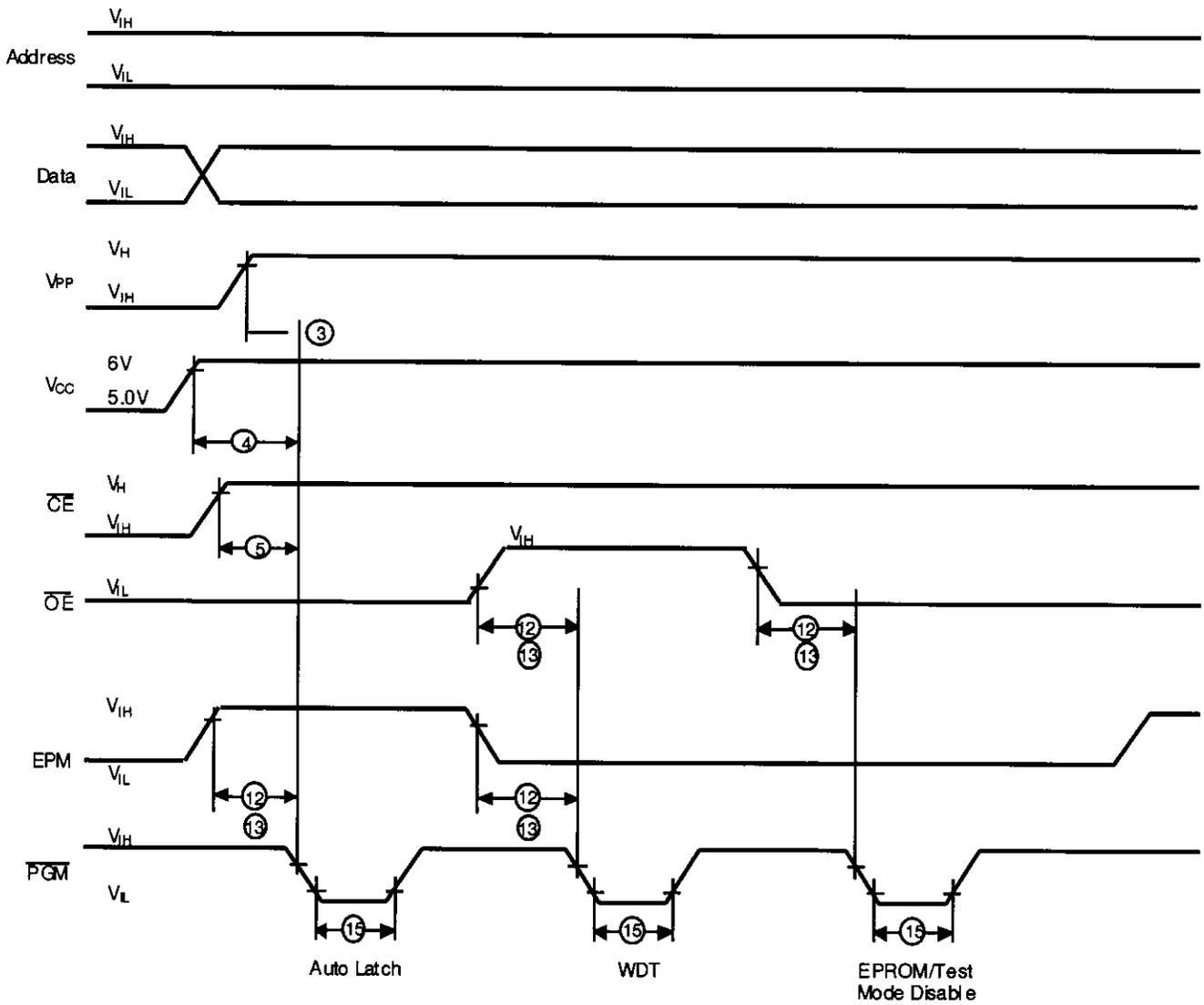
**Figure 22. Z86E04/E08 Programming Options Waveform
