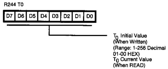
Figure 27. Counter/Timer 0 Register (F4<sub>H</sub>: Read/Write)
