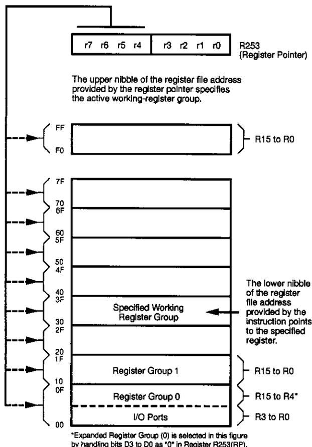
Figure 13. Register Pointer
