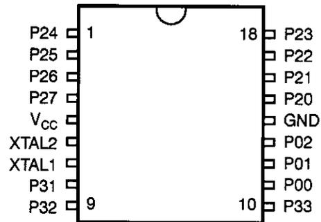
Figure 4. 18-Pin DIP/SOIC Mode Configuration
