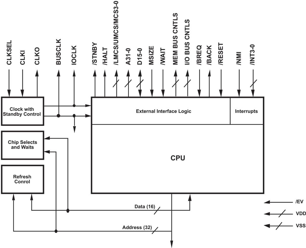
Figure 1. Z380 Functional Block Diagram
