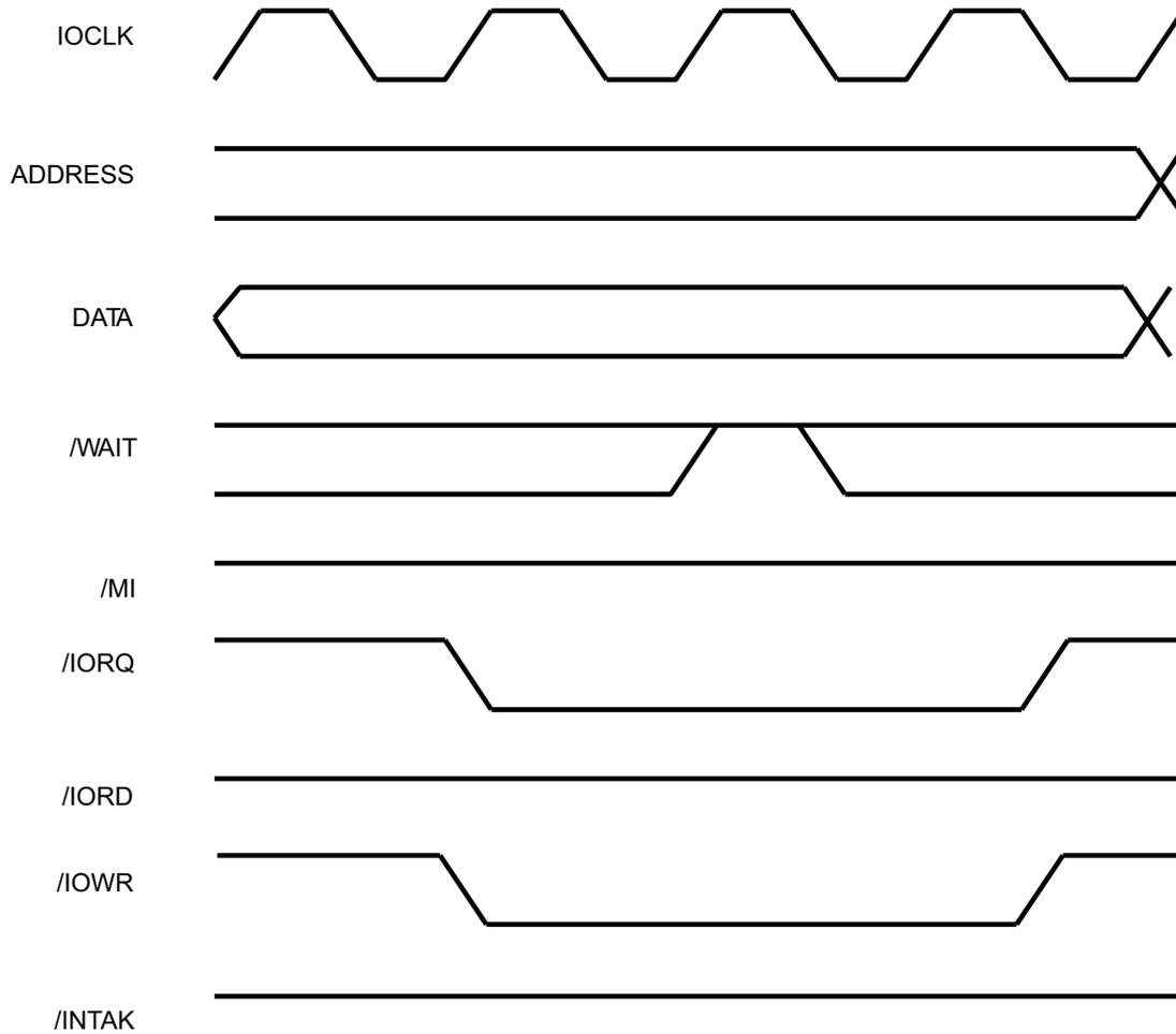
Figure 19. I/O Write Cycle, No Waits
