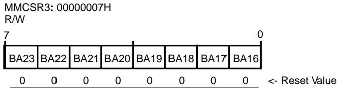
**Figure 39. Mid-range Memory Chip Select Register 3**
