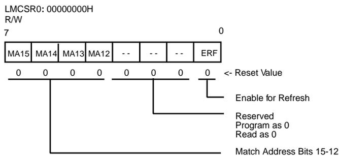
Figure 32. Lower Memory Chip Select Register 0
