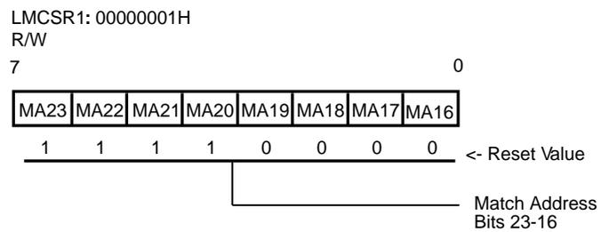
Figure 33. Lower Memory Chip Select Register 1
