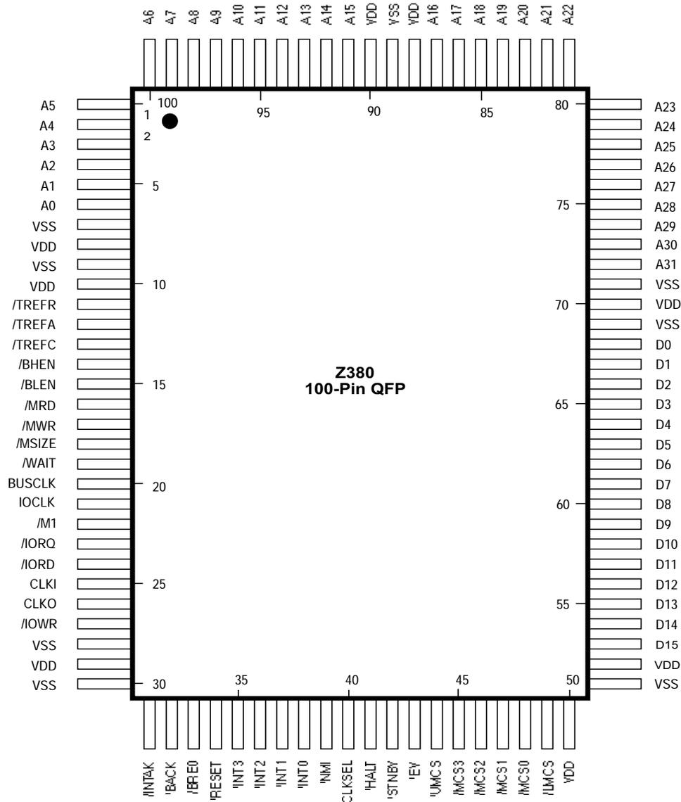
Figure 2. 100-Pin QFP Pin Assignments
