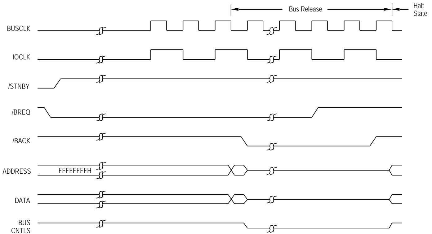
**Figure 52. Standby Mode Exit with Bus Request Timing**
