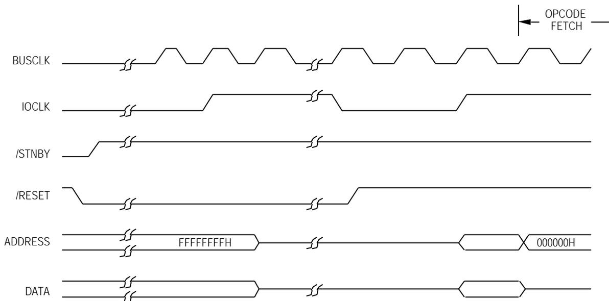
**Figure 54. Standby Mode Exit with Reset Timing**
