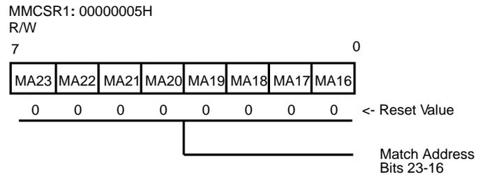
Figure 37. Mid-range Memory Chip Select Register 1
