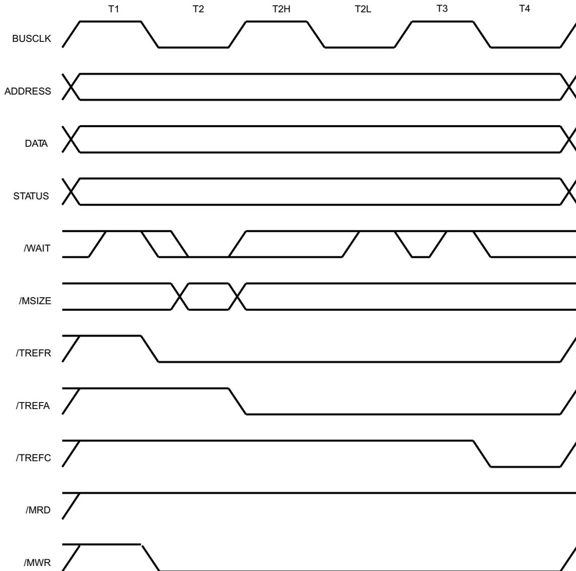
Figure 9. Write Cycle, T2 Wait
