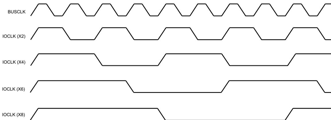
Figure 16. IOCLK Timing
