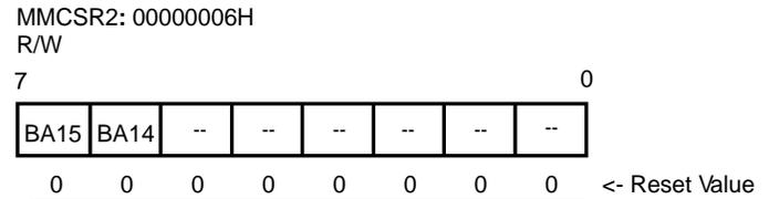
Figure 38. Mid-range Memory Chip Select Register 2
