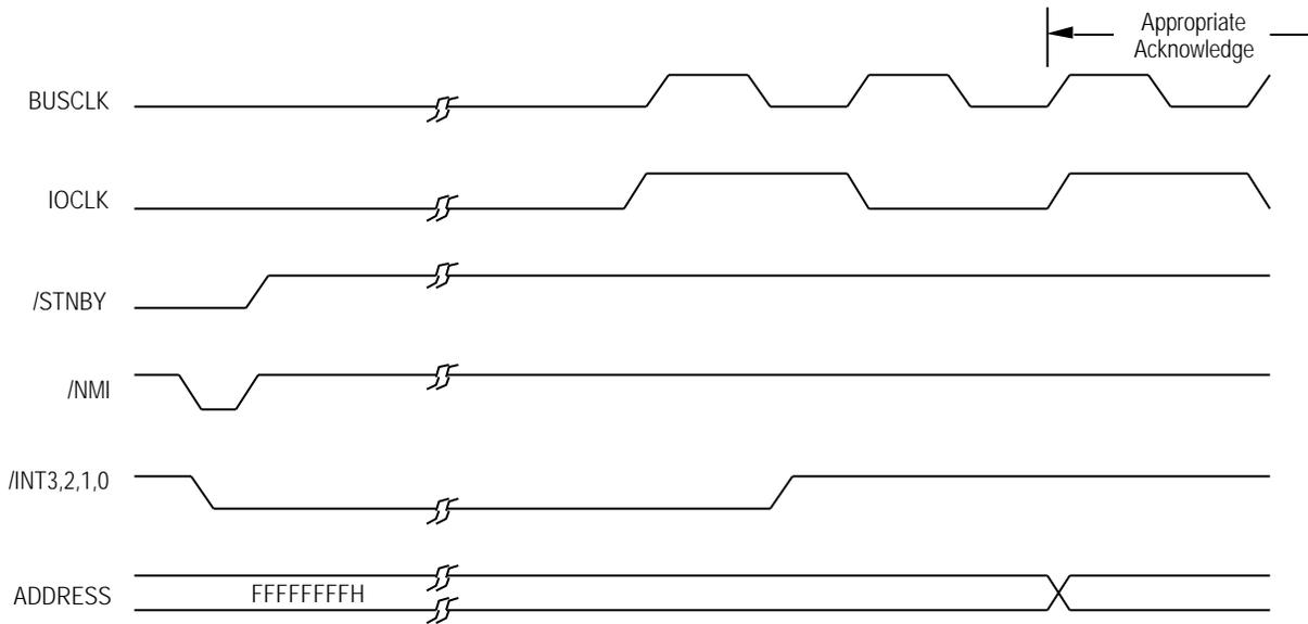
**Figure 55. Standby Mode Exit with External Interrupts Timing**
