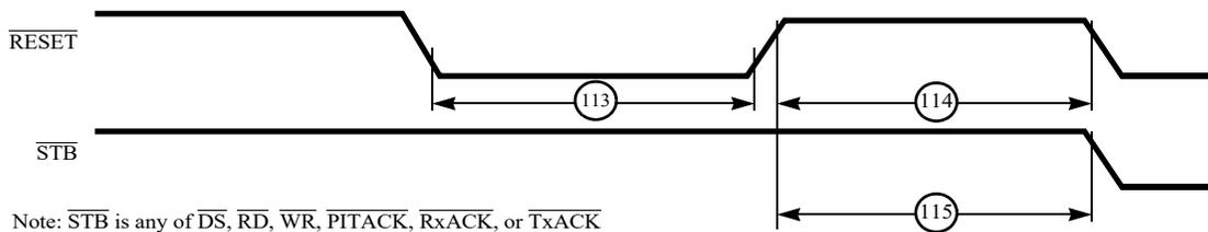
**Figure 6. Reset Timing**
