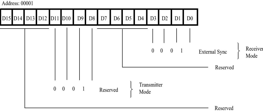
Figure 33. Channel Mode Register, External Sync Mode
