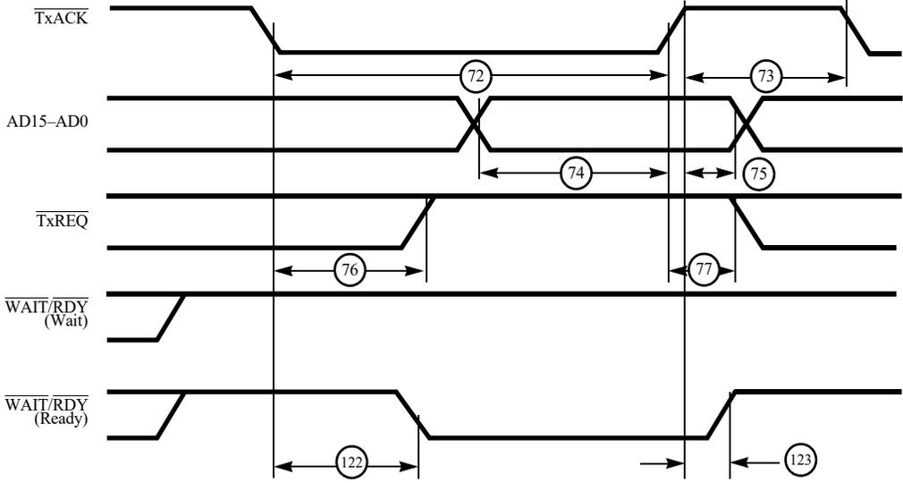
Figure 9. DMA Write Cycle
