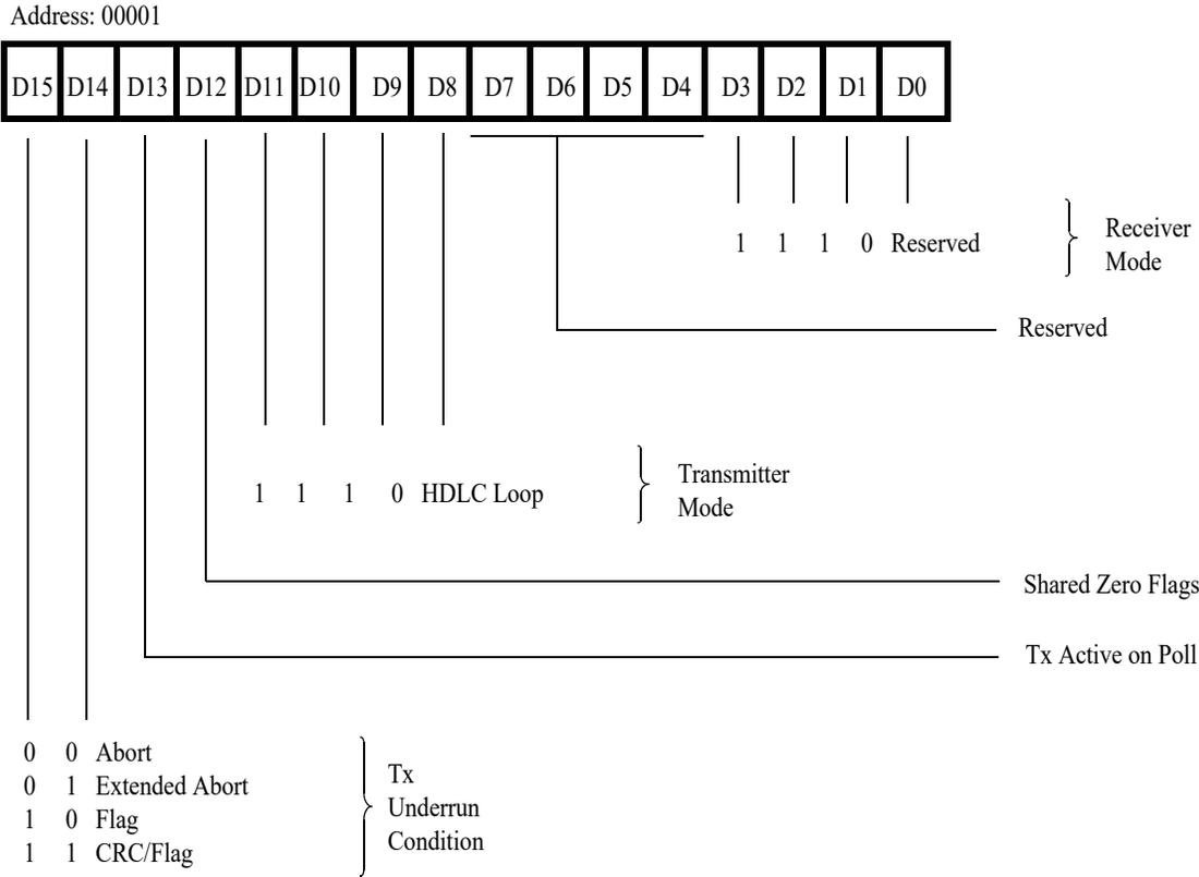
Figure 43. Channel Mode Register, HDLC Loop Mode
