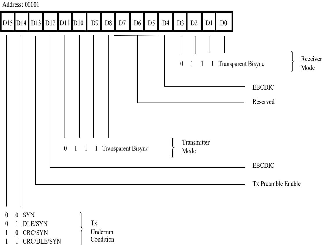
**Figure 39. Channel Mode Register, Transparent Bisync Mode**
