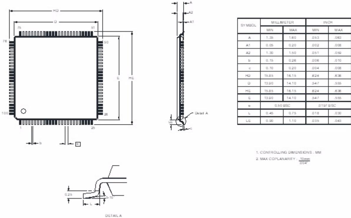
Figure 78. 100-Pin LQFP Package Diagram
