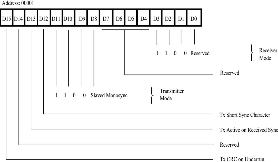
Figure 42. Channel Mode Register, Slaved Monosync Mode
