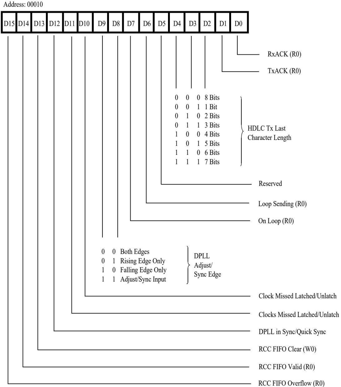
Figure 44. Channel Command/Status Register
