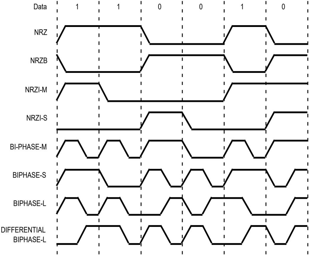
Figure 28. Data Encoding
