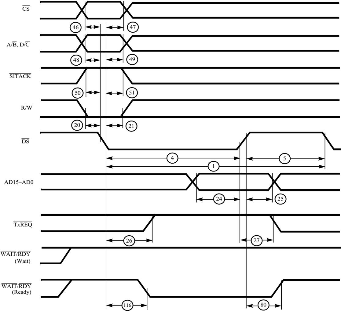
Figure 15. Nonmultiplexed  $\overline{DS}$  Write Cycle
