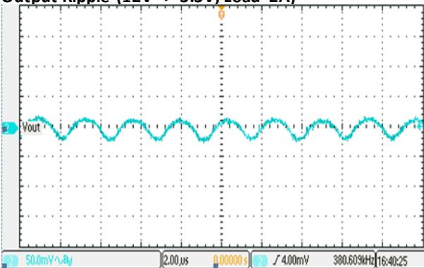
**Output Ripple (12V => 3.3V, Load=1A)**
