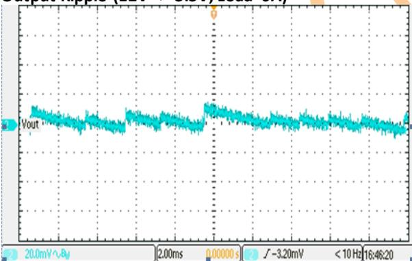
**Dynamic Load ( $I_{load}=0.5A$  2A  $V_{out}=3.3V$ )**
