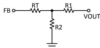
Figure 4: Structure of the feedback circuit.
