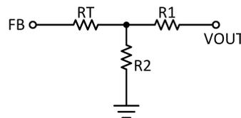
Figure 4: Structure of the feedback circuit.
