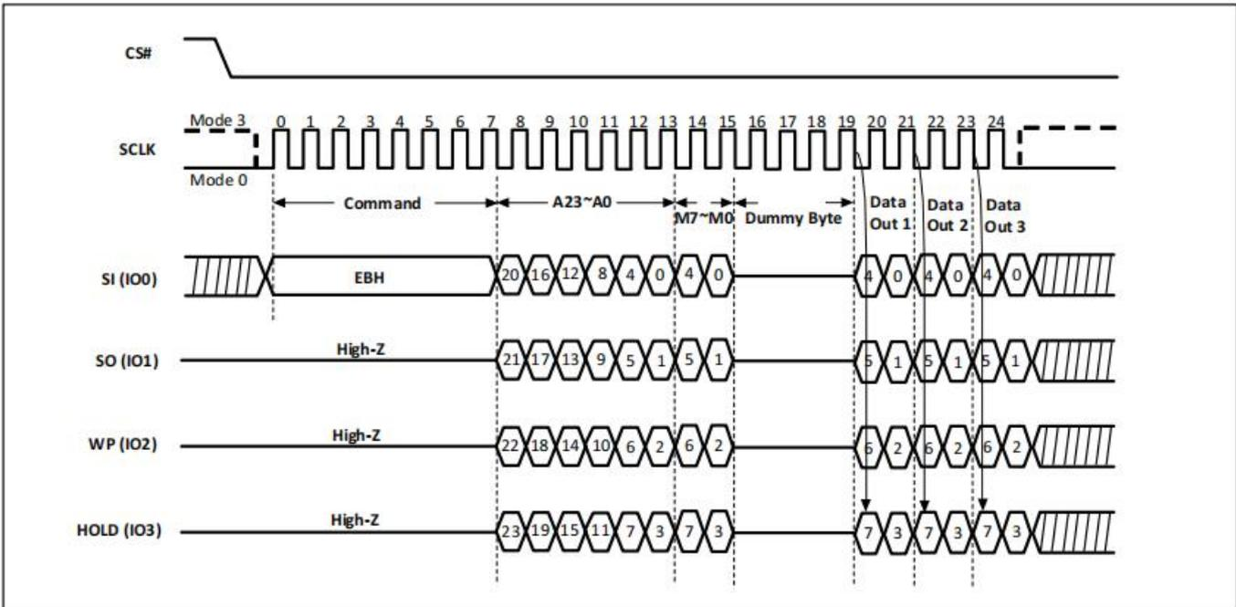
**9.14 Quad I/O Fast Read with “Continuous Read Mode” (EBH)**
