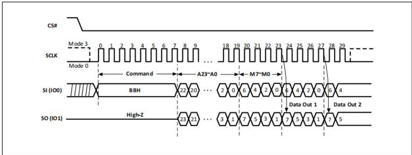
**9.11 Dual I/O Fast Read with “Continuous Read Mode” (BBH)**
