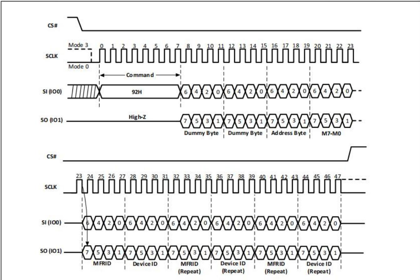
**Note:** The “Continuous Read Mode” bits (M5-4) must be set to (1,0) to be compatible with Dual I/O Fast Read command.
