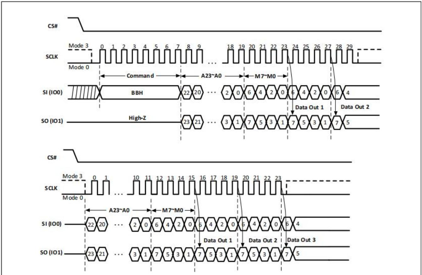
**Note:** Dual I/O Fast Read with “Continuous Read Mode”, if (M5-4)=(1,0). If not using “Continuous Read Mode” recommend setting (M5-4)≠(1,0).
