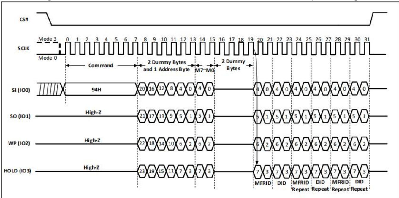
**Note:** The “Continuous Read Mode” bits (M5-4) must be set to (1,0) to be compatible with Quad I/O Fast Read command.
