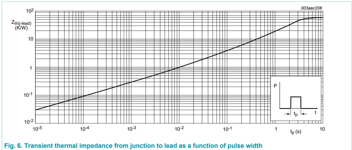
Fig. 6. Transient thermal impedance from junction to lead as a function of pulse width
