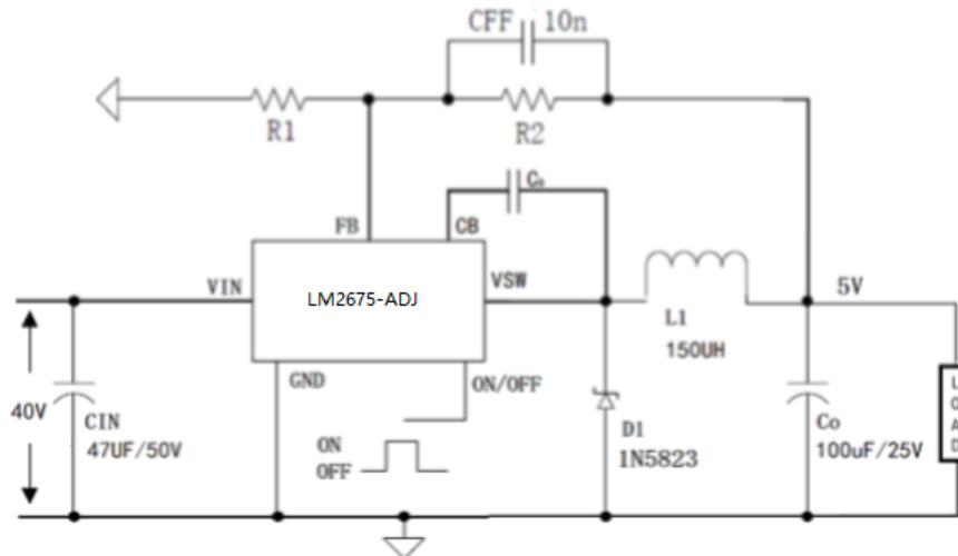
$$V_{OUT} = V_{REF} (1 + R2/R1)$$
