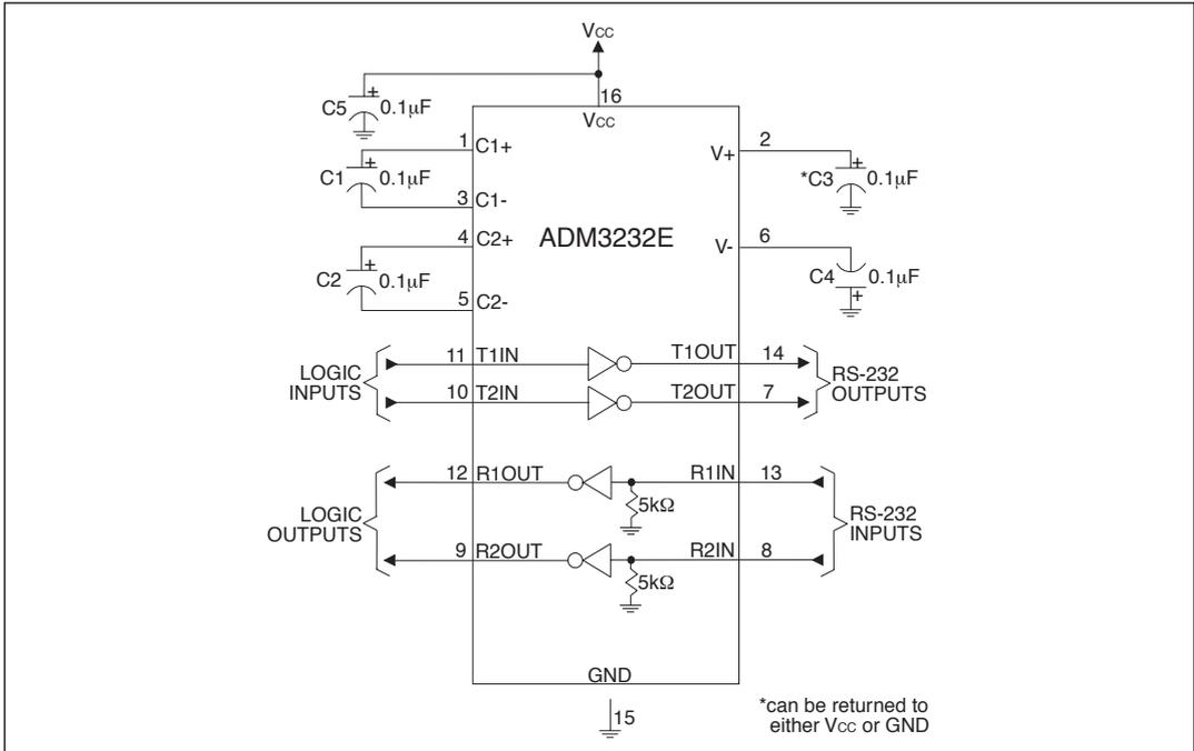
Figure 7. ADM3232E Typical Operating Circuit
