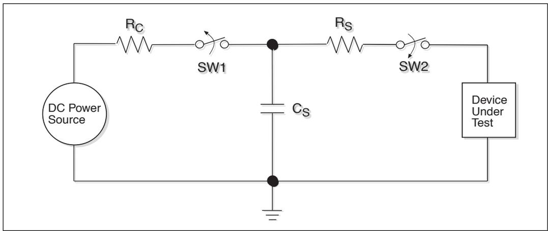
Figure 17. ESD Test Circuit for Human Body Model
