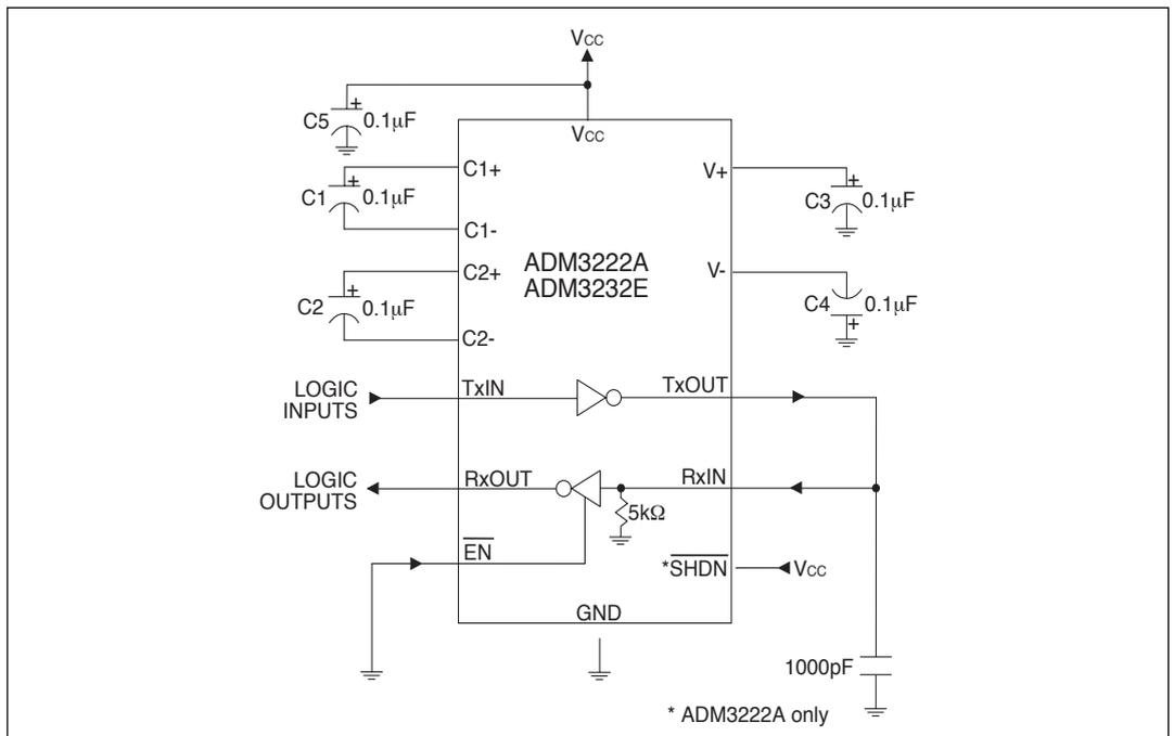
Figure 8. ADM3222A/3232E Driver Loopback Test Circuit
