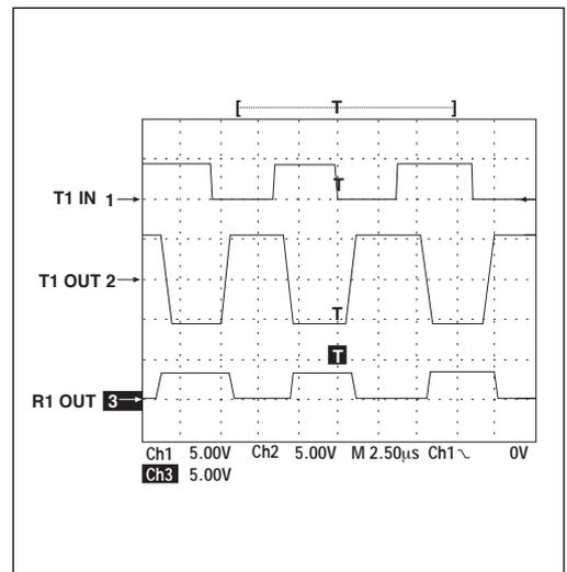
Figure 10. Driver Loopback Test Results at 235kbps
