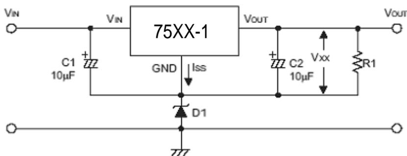
$$V_{OUT} = V_{XX} + VD1$$
