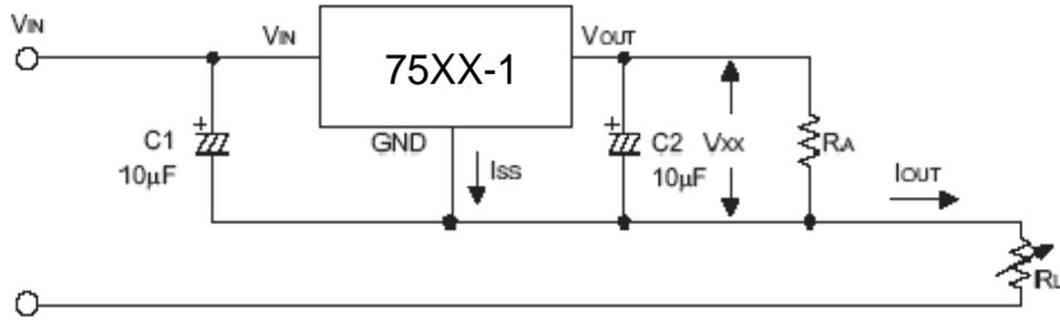
$$I_{OUT} = V_{XX}/R_X + I_{SS}$$
