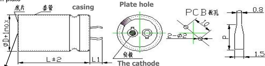
防爆筋(Explosion-proof reinforcement)
