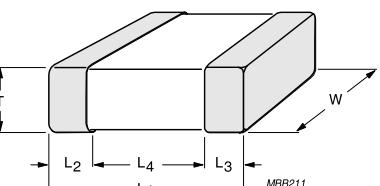
Fig. 2 Surface mounted multilayer ceramic capacitor dimension
