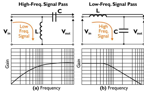
Filtering functions of capacitor coupled with inductor
