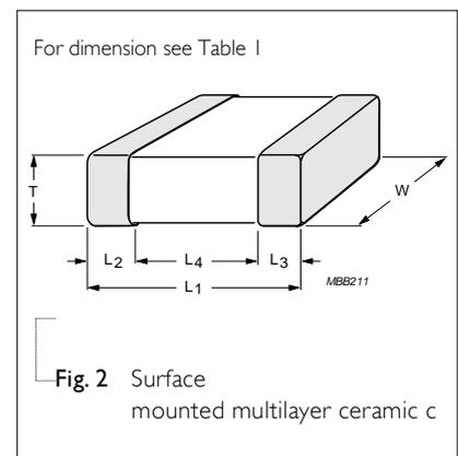
Fig. 2 Surface mounted multilayer ceramic c
