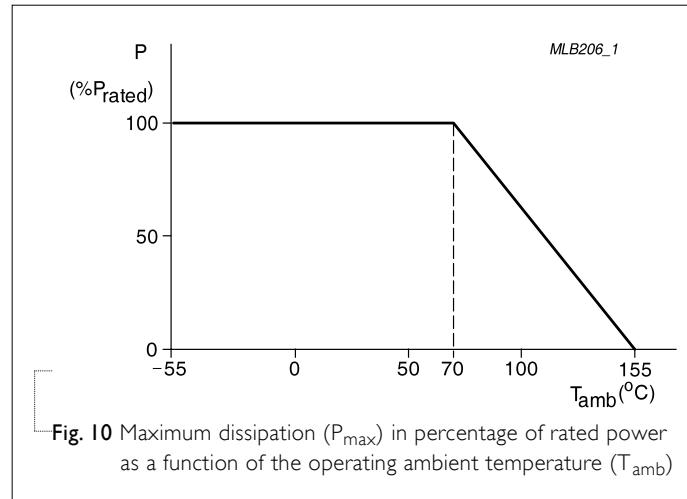
Fig. 10 Maximum dissipation ( $P_{\max}$ ) in percentage of rated power as a function of the operating ambient temperature ( $T_{\text{amb}}$ )
