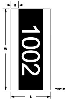
Fig. 4 Chip resistor dimensions
