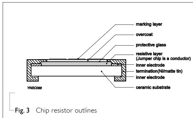
Fig. 3 Chip resistor outlines
