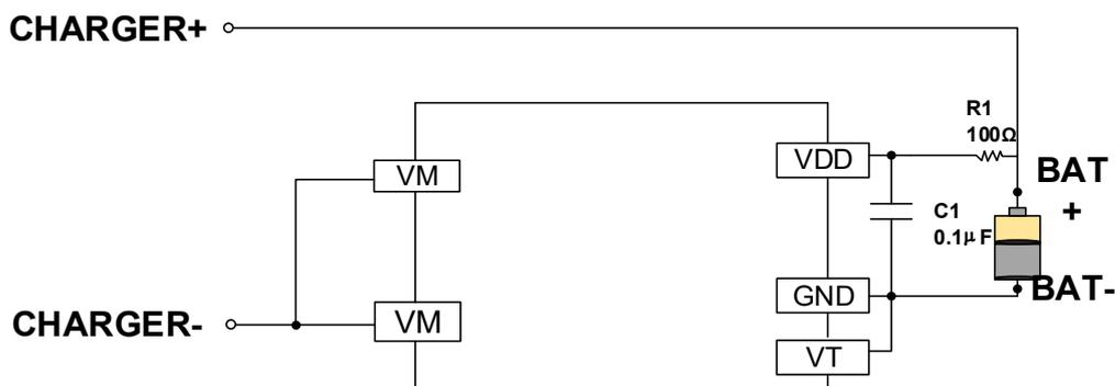
**Figure 5 XB5332B in a Typical Battery Protection Circuit**
