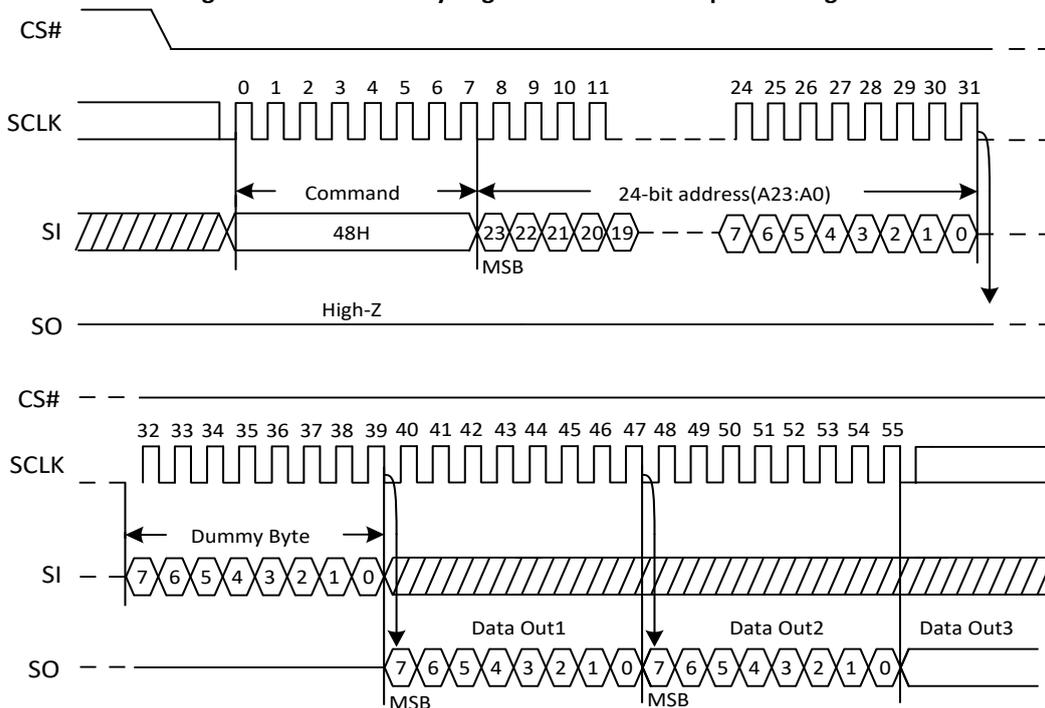
Note: The Byte Address A2-A0 must be 000.
