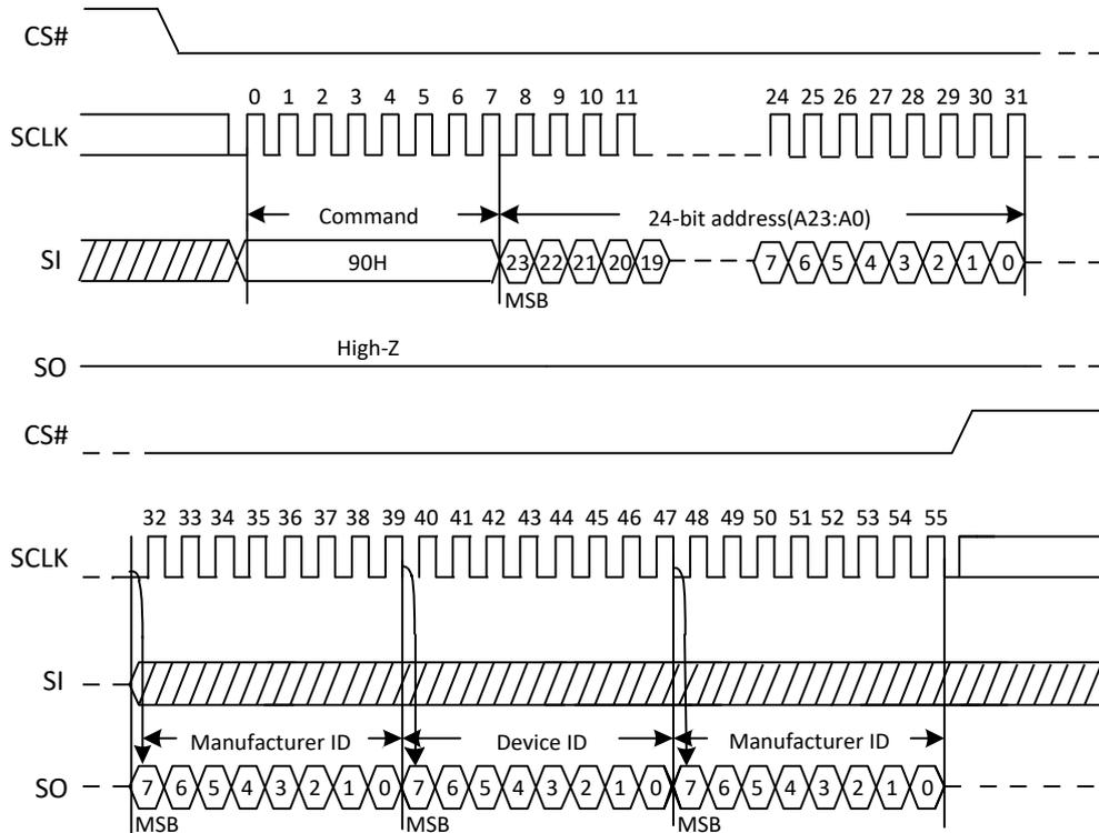
Figure 32a. Read Manufacture ID/ Device ID Sequence Diagram (QPI)
