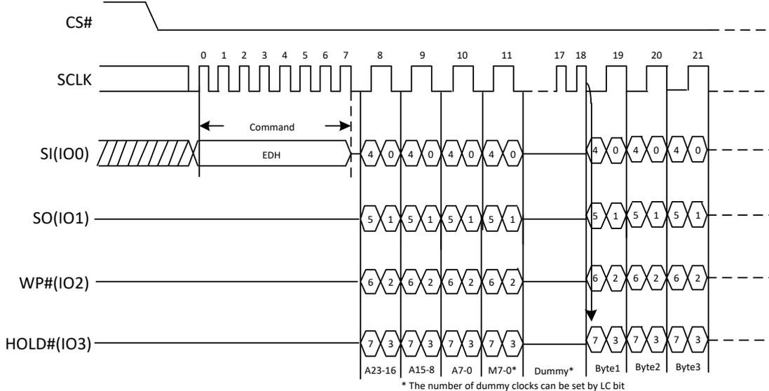
**Figure 17a. Fast Read Quad I/O (Previous instruction set M5-4=10, SPI Mode)**
