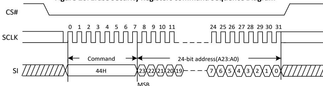
Note: When performing program security register or erase security register, program erase suspend (op code is 75H/B0H) is not allowed, if issuing suspend op code during program or erase security register, the device may enter into malfunction.
