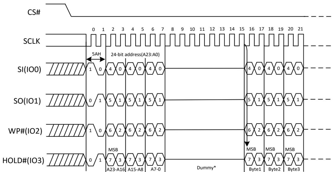
\*Set Read Parameters Command (COH) can set the number of dummy clocks
