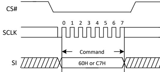
Figure 23a. Chip Erase Sequence Diagram (QPI)
