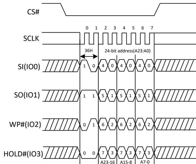
Figure 38b. Individual Block/Sector Unlock command Sequence Diagram
