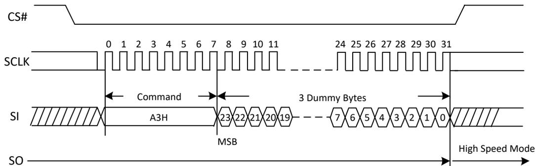
Figure 7a. High Speed Mode Sequence Diagram (QPI)
