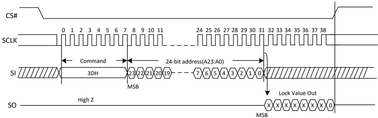
Figure 38e. Read Individual Block/Sector lock command Sequence Diagram (QPI)
