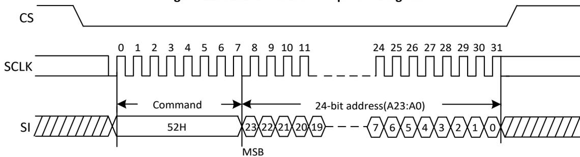
Figure 21a. 32kB Block Erase Sequence Diagram (QPI)
