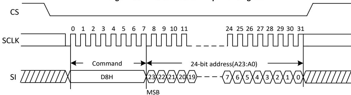
Figure 22a. 64kB Block Erase Sequence Diagram (QPI)
