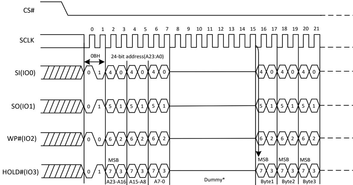
\*Set Read Parameters Command (C0H) can set the number of dummy clocks
