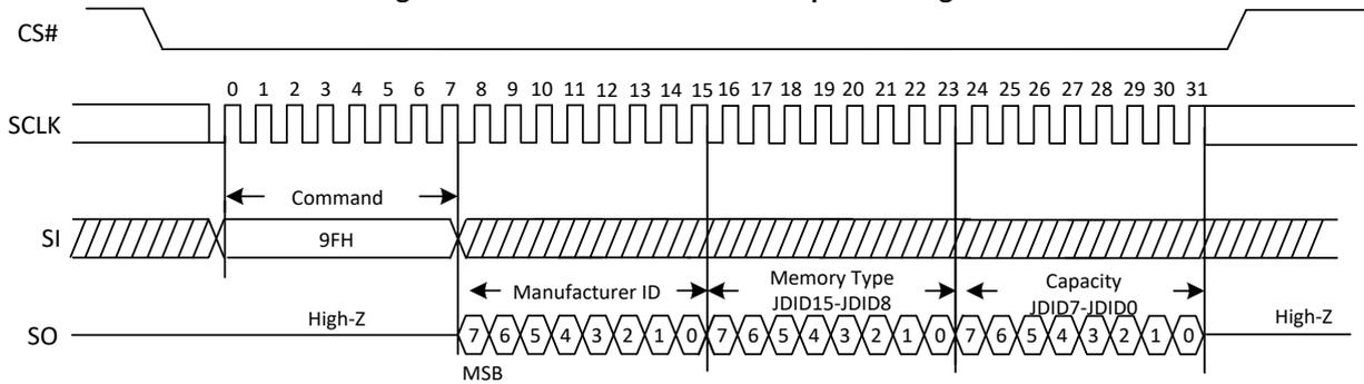
Figure 35a. Read Identification ID Sequence Diagram (QPI)
