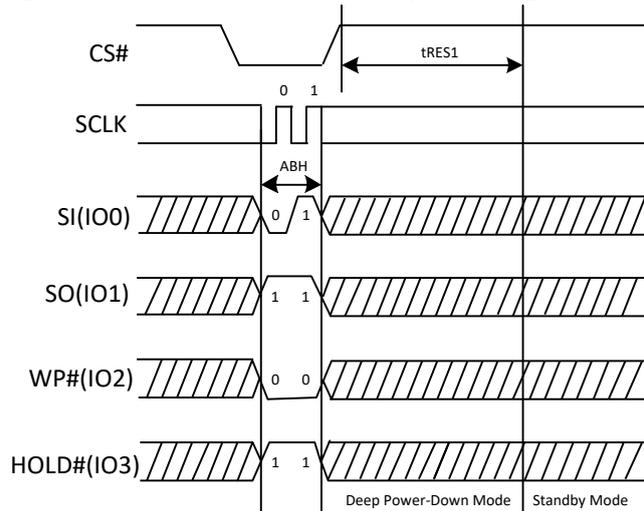
Figure 30b. Release Power-Down/Read Device ID Sequence Diagram
