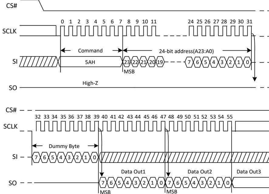
Note: A23-A8 = 0, A7-A0 is the starting byte address for 256-byte SFDP Register.
