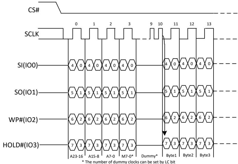
**DTR Fast Read Quad I/O with “8/16/32/64-Byte Wrap Around” in Standard SPI mode**
