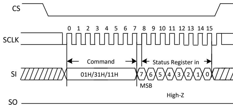
Figure 28a. Write Status Register Sequence Diagram (QPI)
