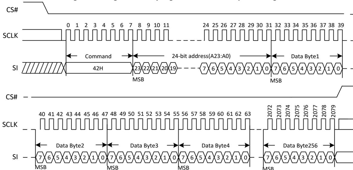
Note: When performing program security register or erase security register, program erase suspend (op code is 75H/B0H) is not allowed, if issuing suspend op code during program or erase security register, the device may enter into malfunction.
