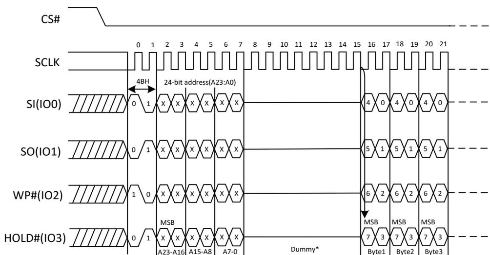
\*Set Read Parameters command (COH) can set the number of dummy cycles
