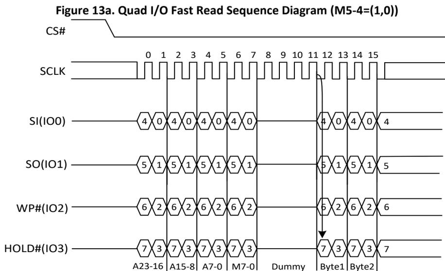
**Quad I/O Fast Read with “8/16/32/64-Byte Wrap Around” in Standard SPI mode**
