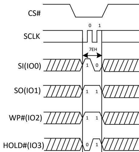
Figure 39b. The Global Block/Sector Unlock Sequence Diagram
