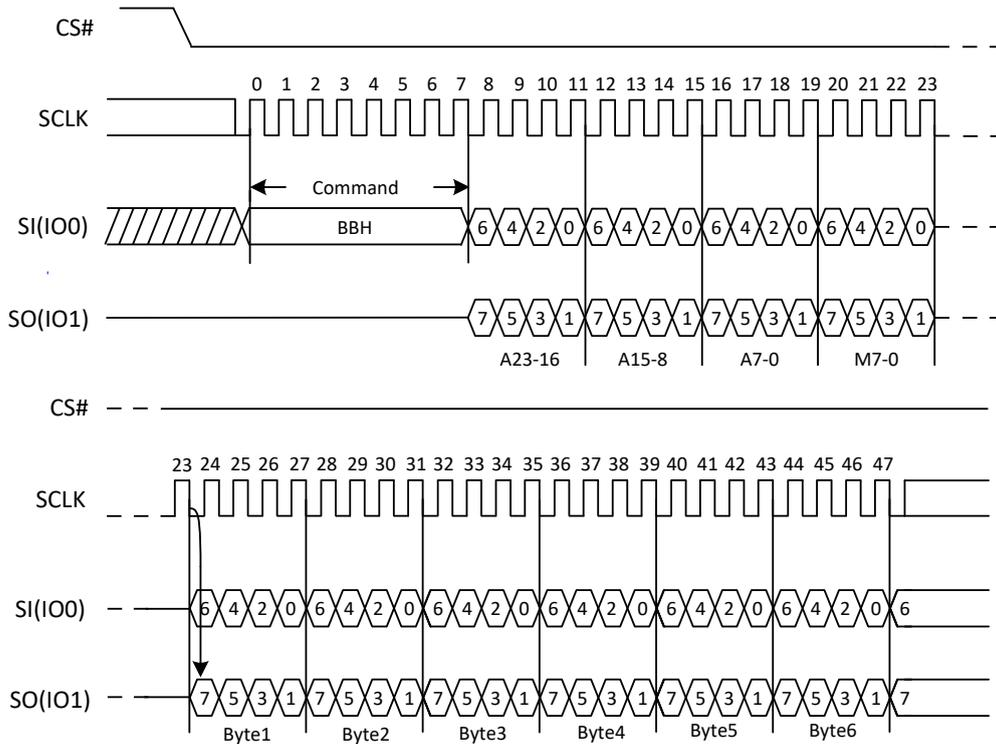
Figure 10a. Dual I/O Fast Read Sequence Diagram (M5-4= (1, 0))
