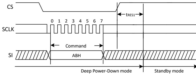
Figure 21a. Release Power-Down/Read Device ID Sequence Diagram
