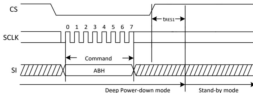
Figure 26. Release Power-Down/Read Device ID Sequence Diagram
