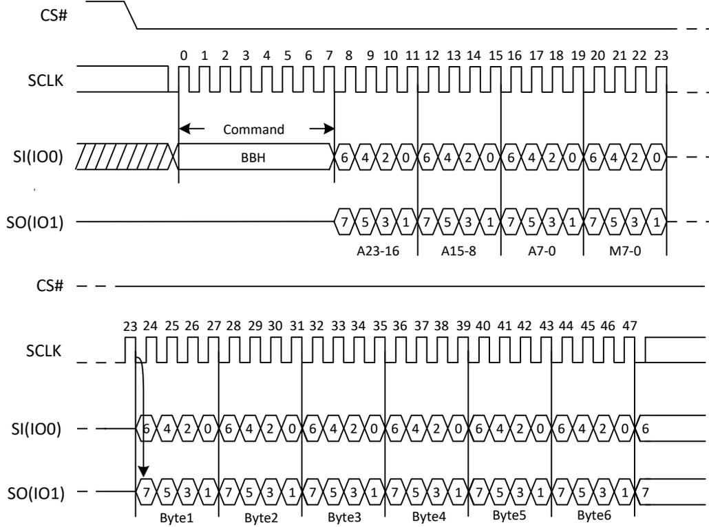
**Figure 12. Dual I/O Fast Read Sequence Diagram (M5-4= (1, 0))**
