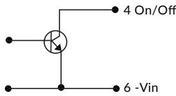
Positive logic: "On" if pin 4 is high >3.5V to 160VDC
