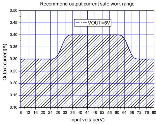
Figure5.Max output current(VOUT=5V)
