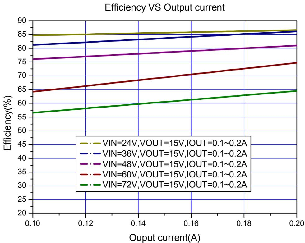
Figure9. XL7005A System Application (Efficiency VS Output Current)
