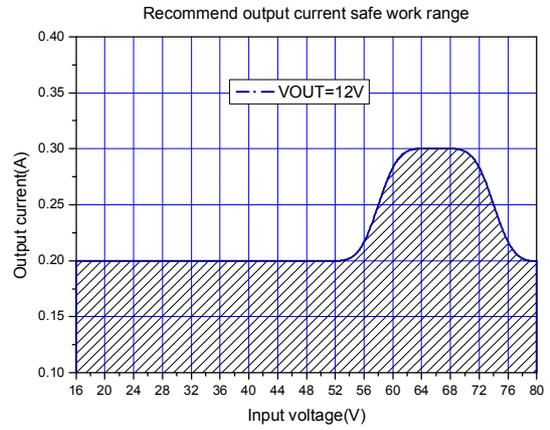
Figure6.Max output current(VOUT=12V)
