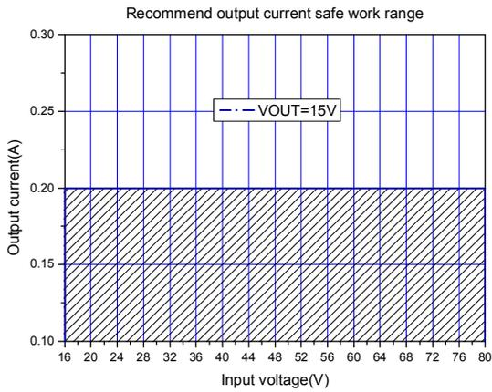
Figure7.Max output current(VOUT=15V)
