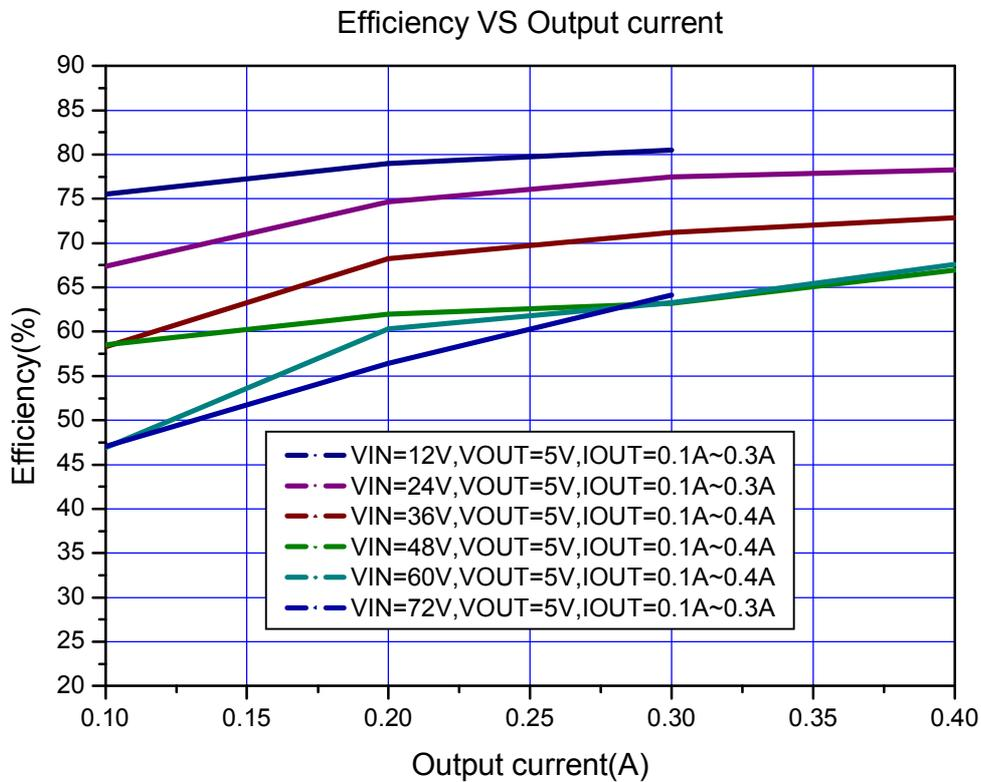
Figure11. XL7005A System Application (Efficiency VS Output Current)
