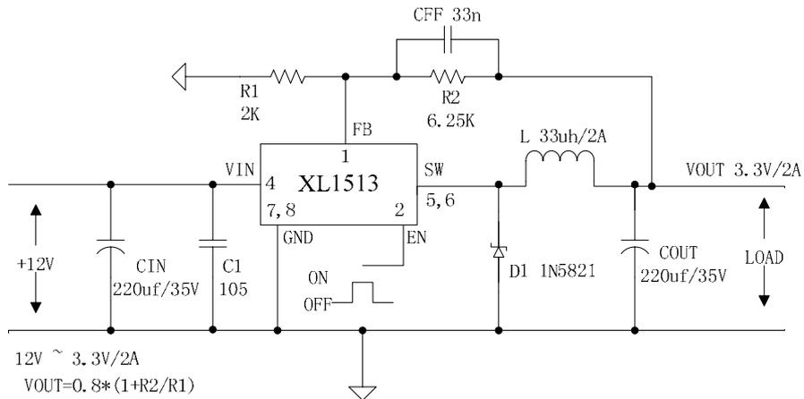
Figure7. XL1513 System Parameters Test Circuit (12V ~ 3.3V/2A)
