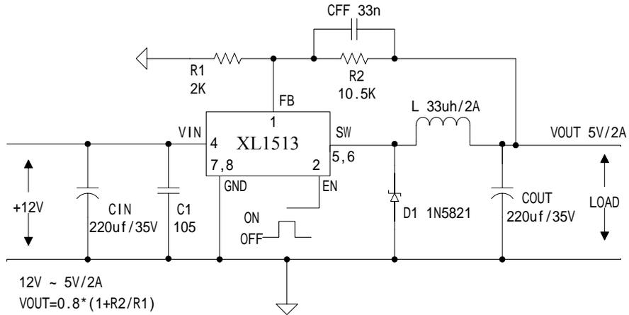
Figure6. XL1513 System Parameters Test Circuit (12V ~ 5V/2A)
