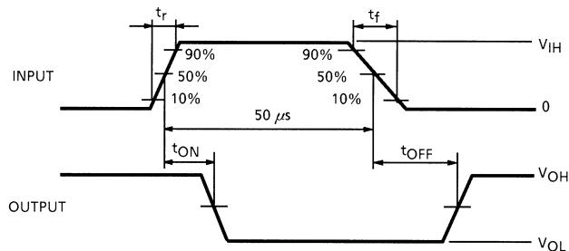
Note 1: Pulse Width 50  $\mu\text{s}$ , Duty Cycle 10%
