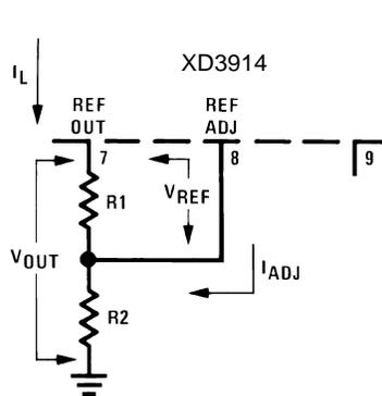
Since the 120 $\mu$ A current (max) from the adjust terminal represents an error term, the reference was designed to minimize changes of this current with  $V^+$  and load changes.
