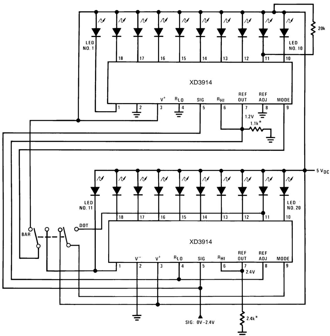
\*The exact wiring arrangement of this schematic shows the need for Mode Select (pin 9) to sense the  $V^+$  voltage exactly as it appears on pin 3.
