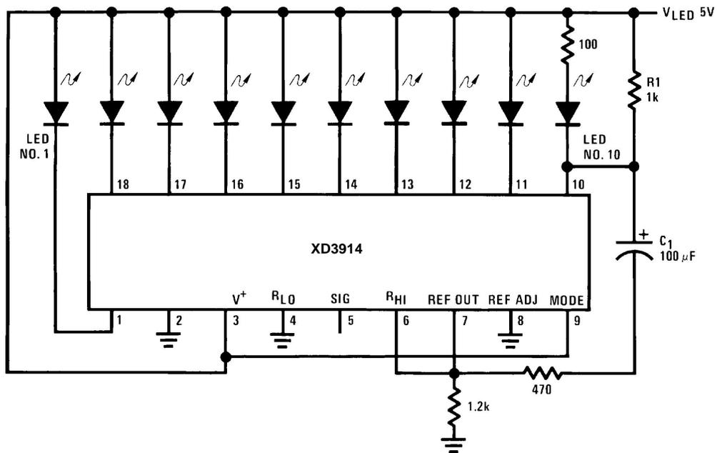
Full-scale causes the full bar display to flash. If the junction of R1 and C1 is connected to a different LED cathode, the display will flash when that LED lights, and at any higher input signal.
