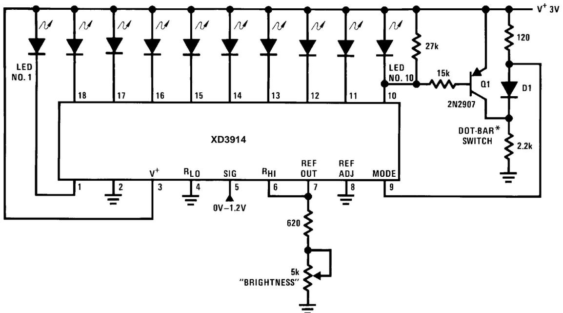
\*The input to the Dot-Bar Switch may be taken from cathodes of other LEDs. Display will change to bar as soon as the LED so selected begins to light.
