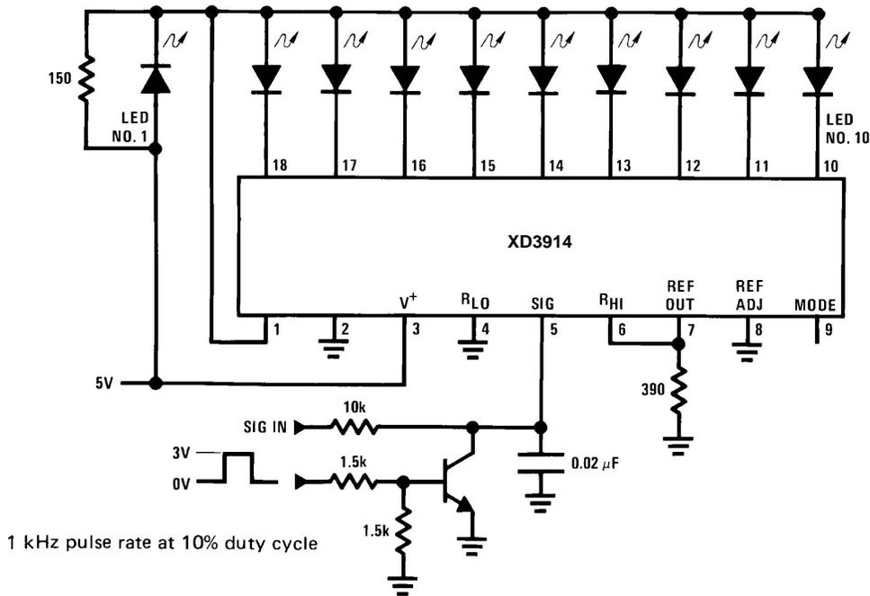
LEDs light up as illustrated with the upper lit LED indicating the actual input voltage. The display appears to increase resolution and provides an analog indication of overrange.
