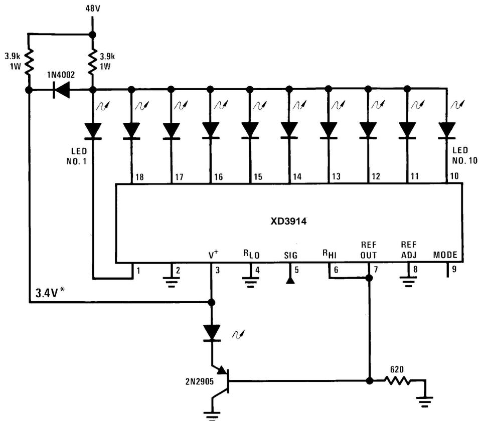
The LED currents are approximately 10mA, and the XD3914 outputs operate in saturation for minimum dissipation.
