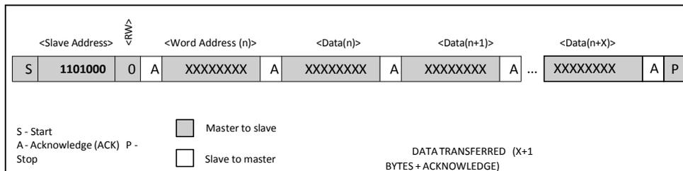
**Figure 6-3. Data Write—Slave Receiver Mode**
