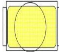
During SMT, please choose the collet that has larger outer diameter than the lighting area of lens, in case that improper position of collet will damage the gold wire inside the LED. Different collets fit for different products, please refer to the following pictures cross out.
