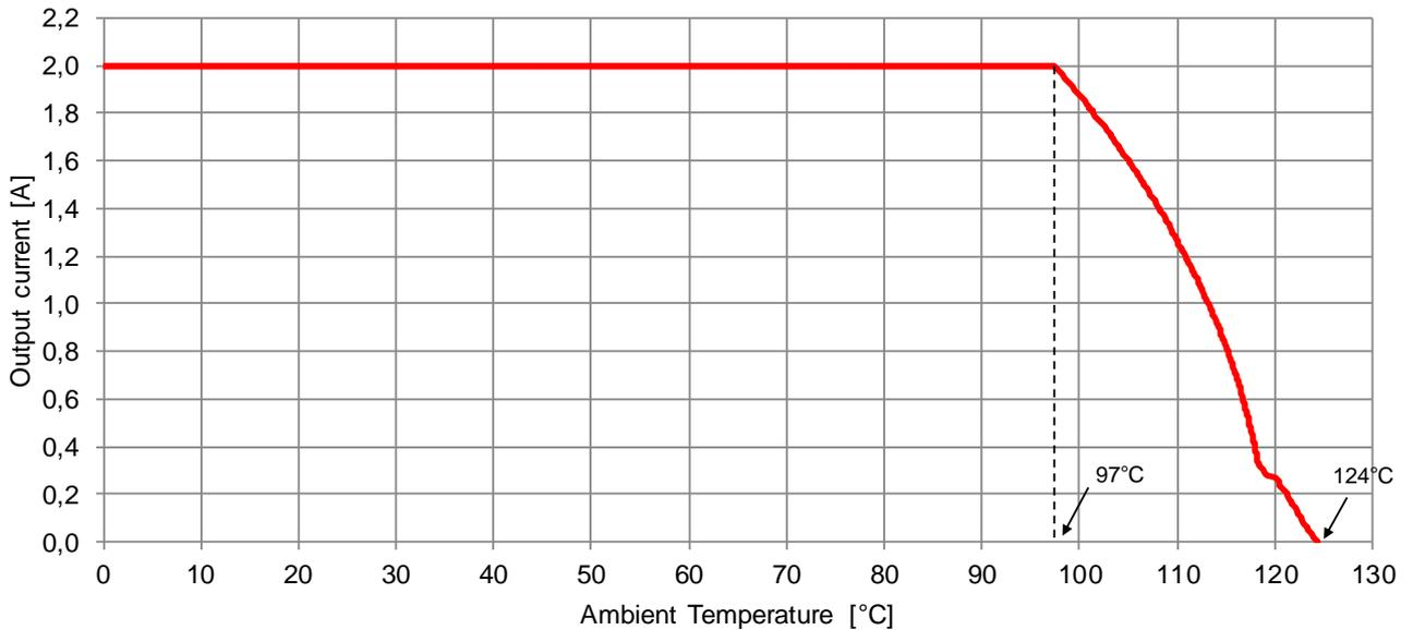
The ambient temperature and the power limits of the derating curve represent the operation at the max junction temperature specified in the "Operating Conditions" section on page 4.
