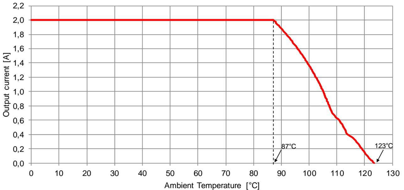
The ambient temperature and the power limits of the derating curve represent the operation at the max junction temperature specified in the "Operating Conditions" section on page 4.
