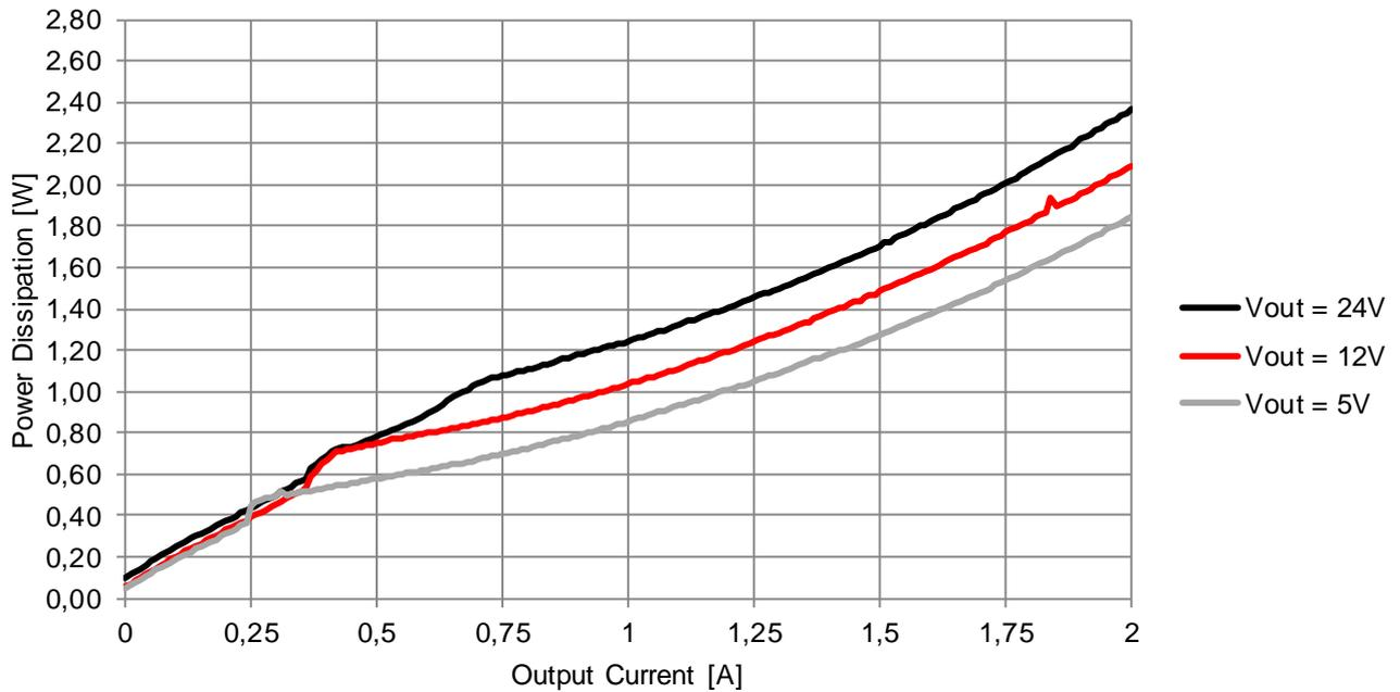
171012402  $V_{IN} = 36V$ ,  $f_{SW} = 500kHz$ ,  $T_A = 85^\circ C$
