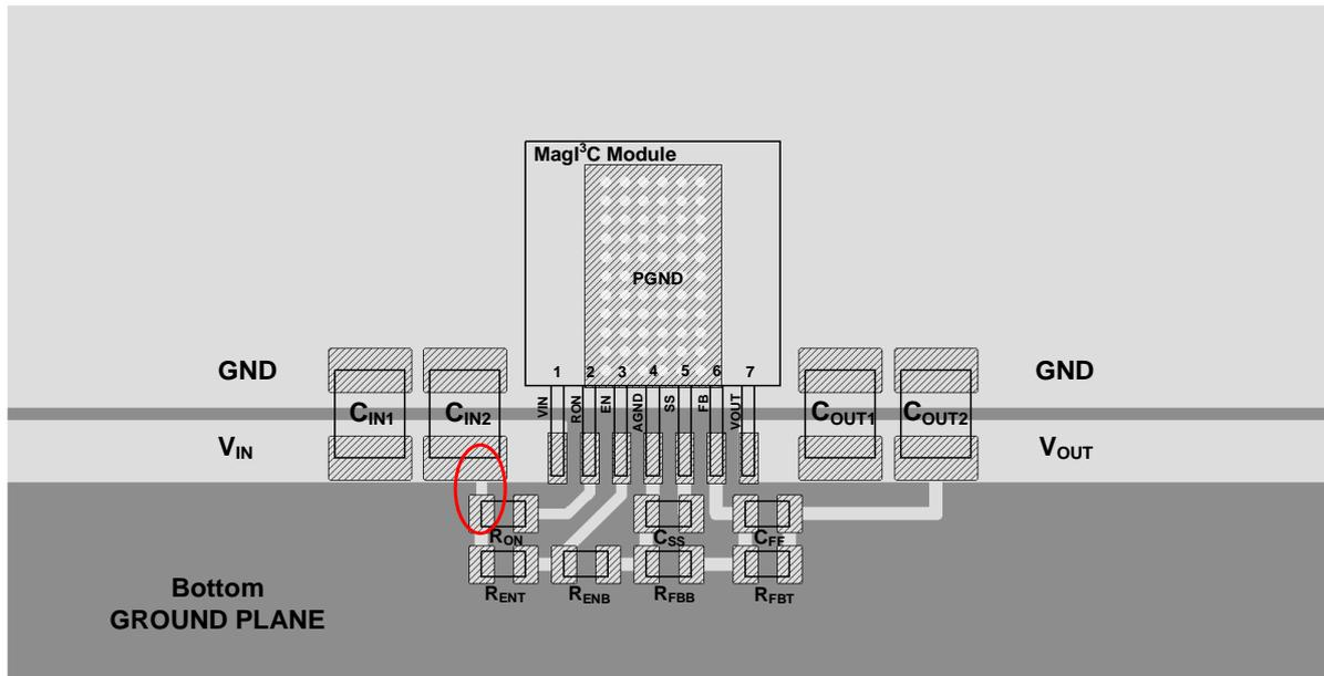
In order to avoid noise injection into RON pin, the resistor  $R_{ON}$  should be routed to one of the input capacitors.
