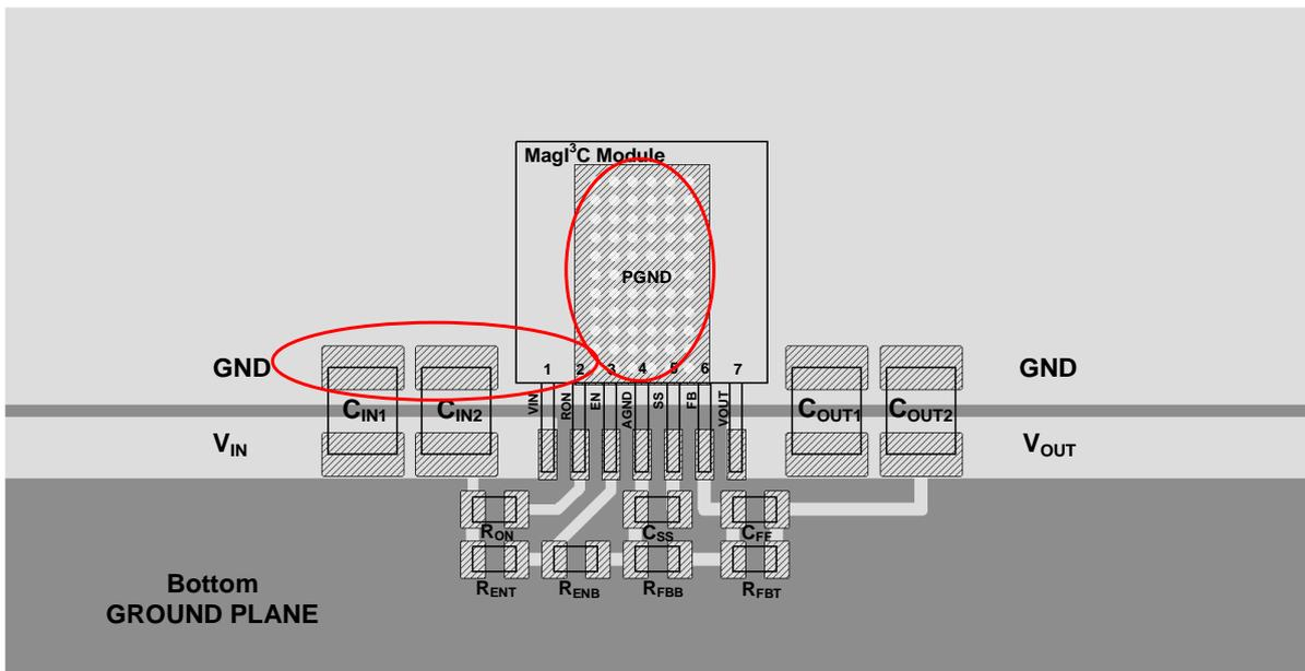
The negative terminal of C<sub>IN1</sub> and C<sub>IN2</sub> needs to be very close to the PGND pad of the power module.
