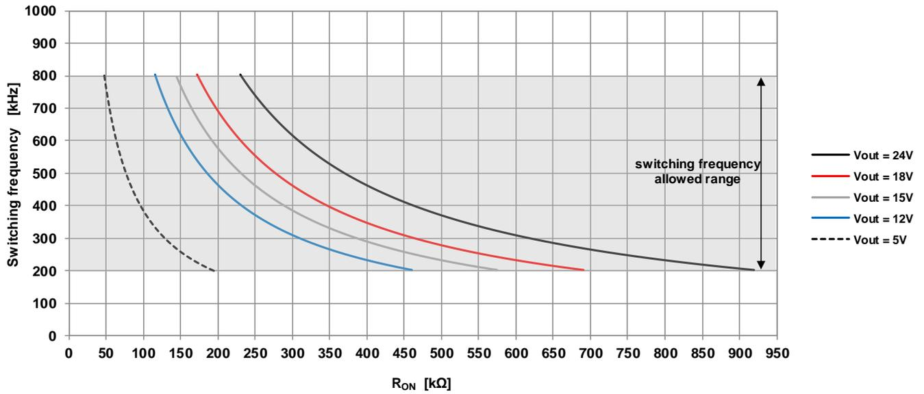
As stated above, the off-time is also limited to a minimum value of 260 ns, which limits the maximum duty cycle. Larger  $R_{ON}$  (lower  $F_{SW}$ ) should be selected in any application requiring large duty ratio.
