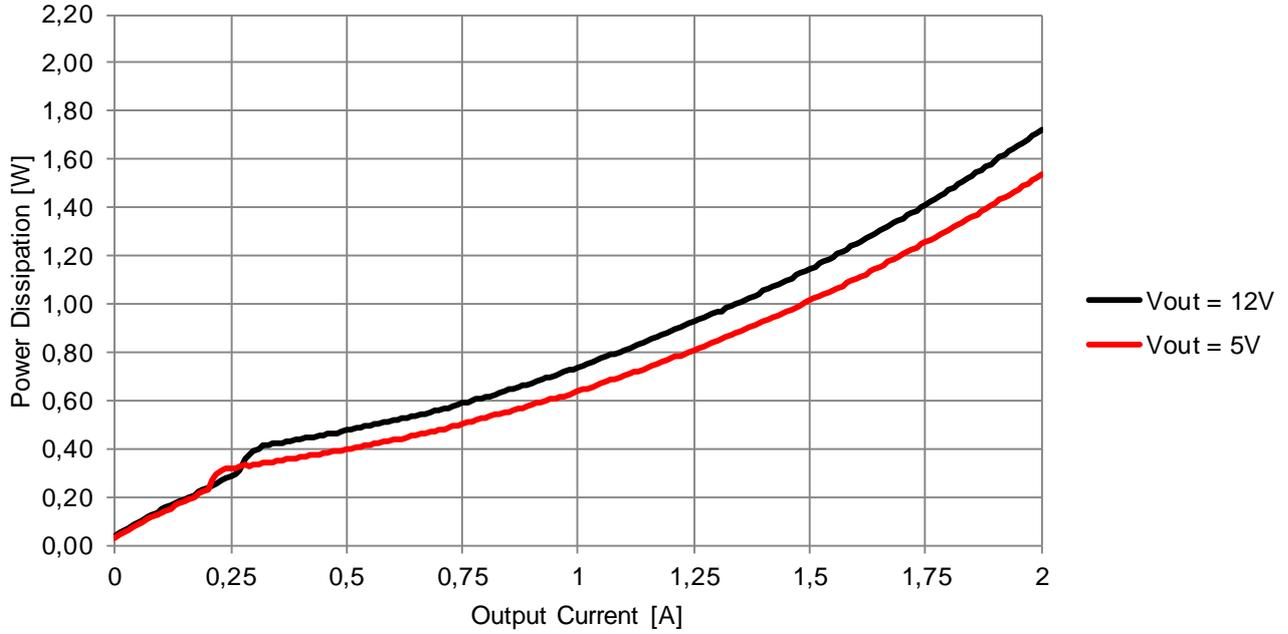
171012402  $V_{IN} = 24V$ ,  $f_{SW} = 500kHz$ ,  $T_A = 85^\circ C$
