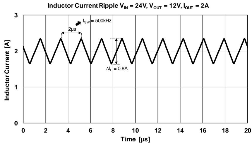
The load current where the transition between DCM and CCM takes place can be estimated using the following formula:
