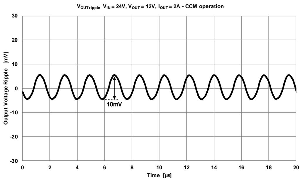
The output voltage ripple during CCM operation is much lower ( $\leq 10mV_{pp}$ ) than the ripple during DCM operation (around  $27mV_{pp}$ ).
