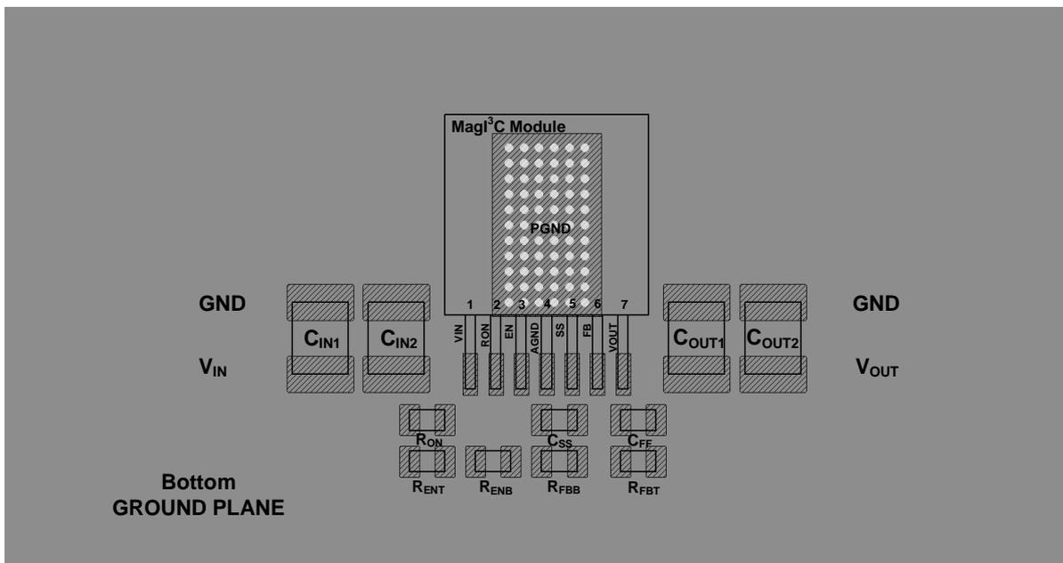
Place a dedicated solid GND copper area beneath the MagI<sup>3</sup>C Power Module.
