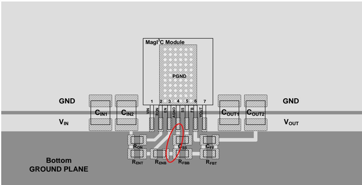
The ground connections for the soft-start capacitor ( $C_{SS}$ ), the output voltage lower resistor divider ( $R_{FBB}$ ) and enable components (when used) should be routed to the AGND pin of the device. If not properly handled, poor grounding can result in degraded load regulation or erratic output voltage ripple behavior. Place  $C_{SS}$ ,  $R_{FBT}$  and  $R_{FBB}$  close to their respective pins.
