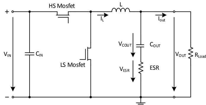
None of the required output capacitors are integrated within the module. A general recommendation in order to guarantee a stable behavior is to place at least a capacitance of 10µF (MLCC recommended) at the output. The output capacitor must meet the worst case RMS current rating, as calculated by equation (8):
