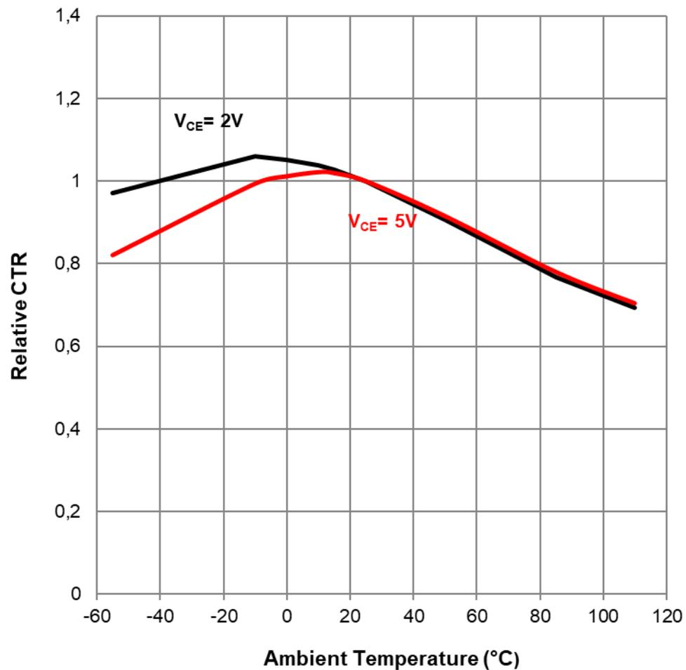
Testcondition: I<sub>F</sub> = 1 mA; normalized to T<sub>A</sub> = 25 °C
