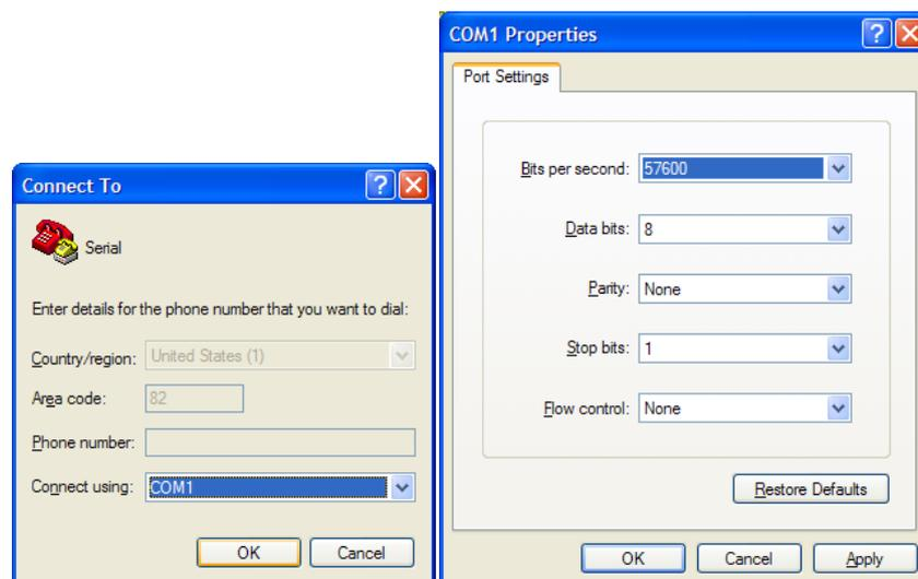
Figure 17. Serial Terminal Program configuration
