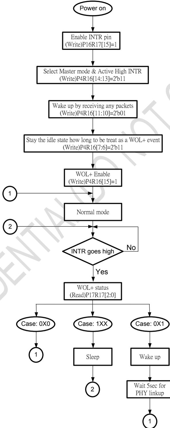
Figure 14 Sleep or wake up automatically programming guide
