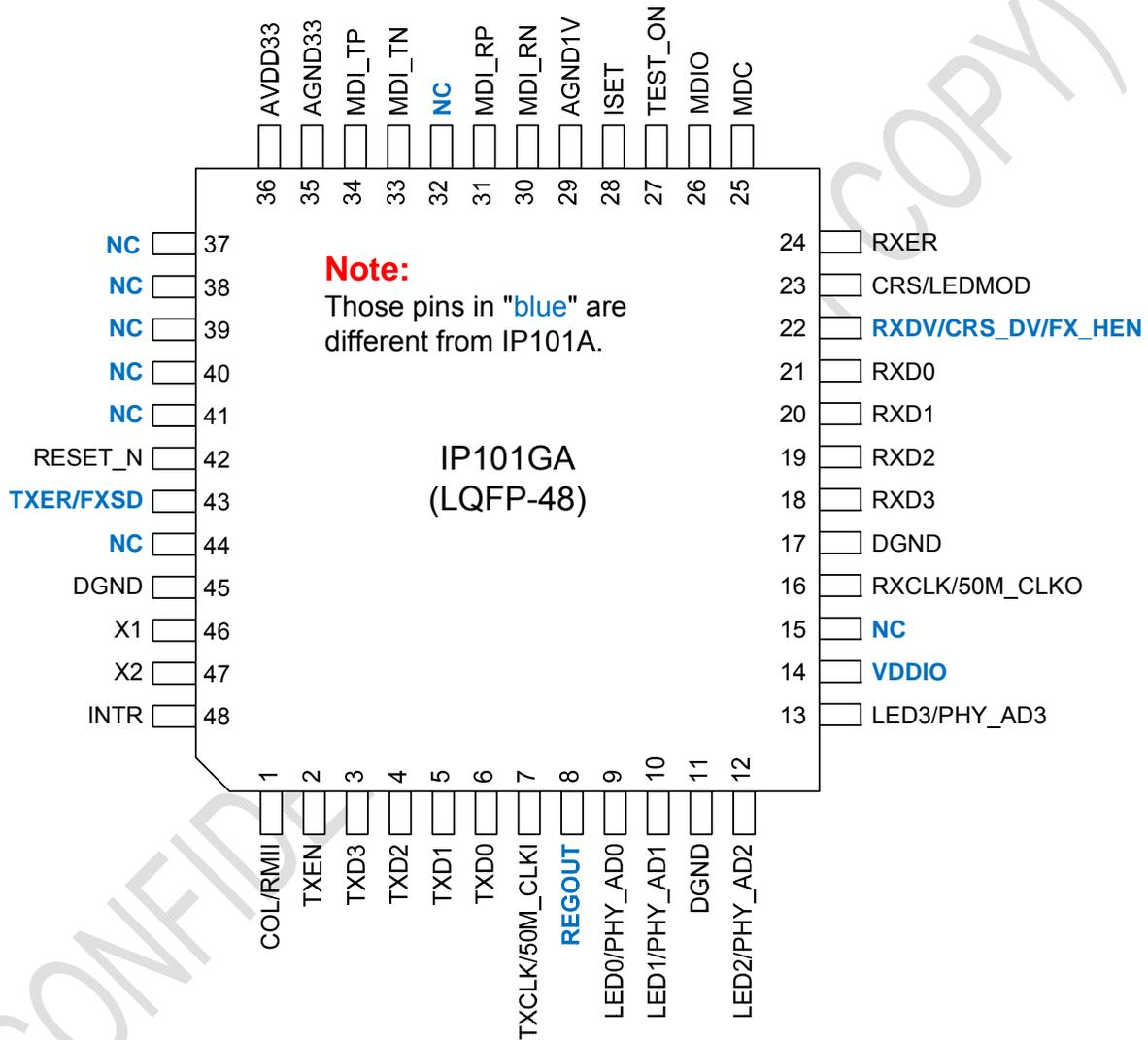
Figure 2 IP101GA 48 Pin Diagram
