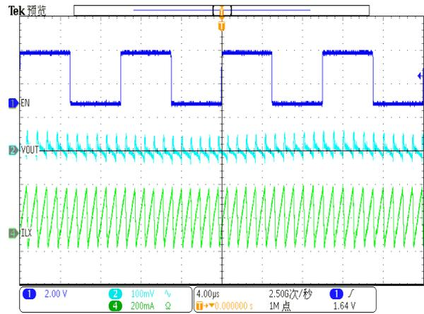
**PWM Dimming Waveforms**
