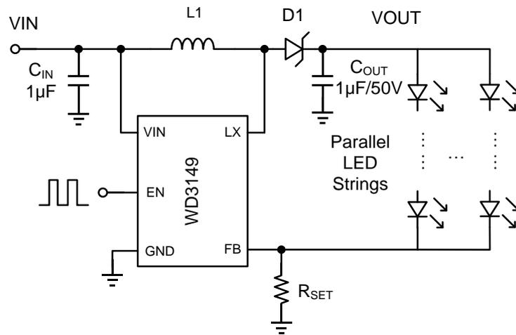
**Figure 7, Li-Ion Driver for Parallel White LED Strings**
