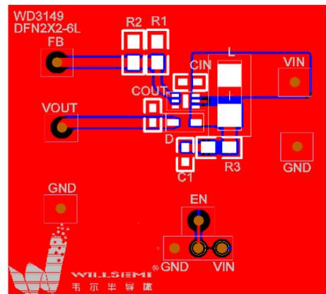
**Figure 4, WD3149 PCB Layout with Snubber**
