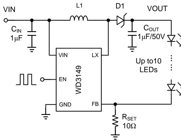
**Figure 5, Li-Ion Driver for 10-S White LEDs**
