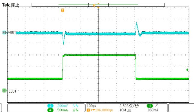
Load Transient;  $V_{IN}=28V, V_{EN}=5V, V_{OUT}=5V, I_{OUT}=0.5A-1.5A$
