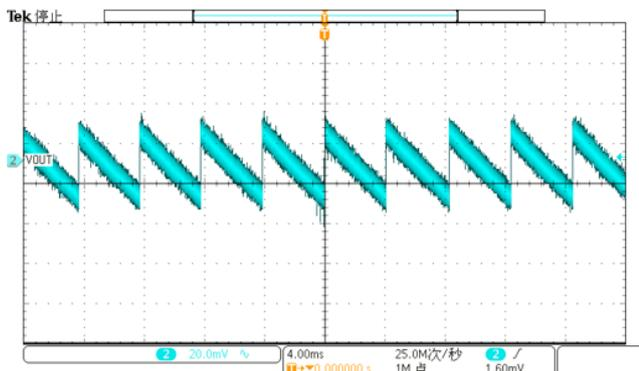
Ripple;  $V_{IN}=12V$ ,  $V_{EN}=5V$ ,  $V_{OUT}=5V$ ,  $I_{OUT}=0mA$
