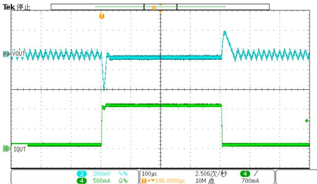
Load Transient;  $V_{IN}=12V, V_{EN}=5V, V_{OUT}=5V, I_{OUT}=0.1A-1A$
