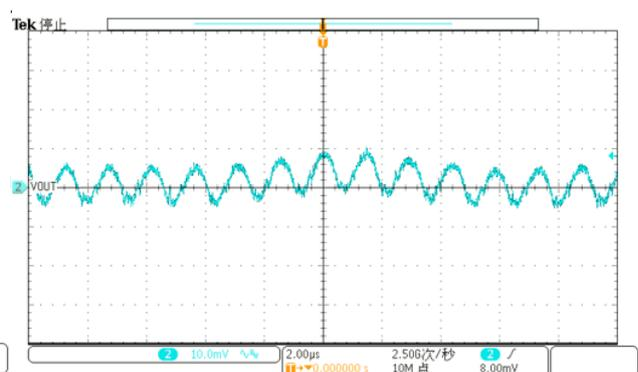
Ripple;  $V_{IN}=12V$ ,  $V_{EN}=5V$ ,  $V_{OUT}=3.3V$ ,  $I_{OUT}=2000mA$
