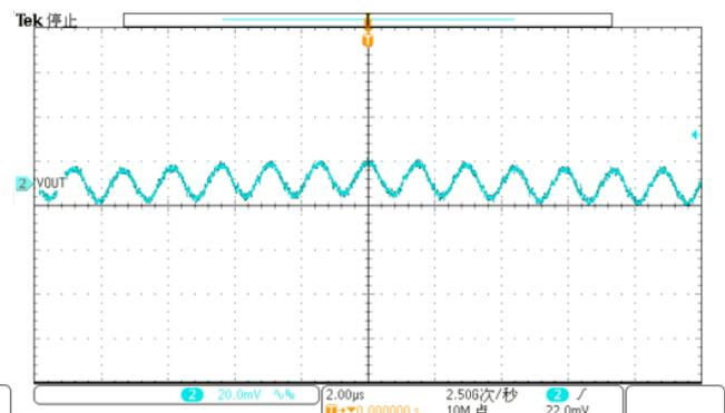
Ripple;  $V_{IN}=12V$ ,  $V_{EN}=5V$ ,  $V_{OUT}=5V$ ,  $I_{OUT}=2000mA$
