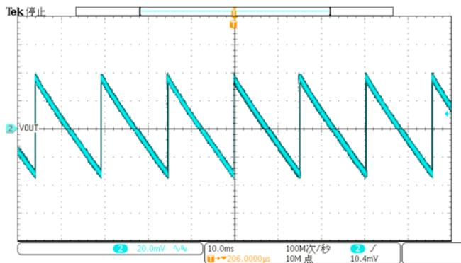
Ripple;  $V_{IN}=12V$ ,  $V_{EN}=5V$ ,  $V_{OUT}=3.3V$ ,  $I_{OUT}=0mA$
