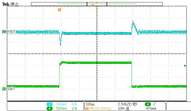
Load Transient:  $V_{IN}=12V, V_{EN}=5V, V_{OUT}=3.3V, I_{OUT}=0.1A-1A$
