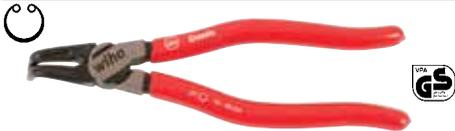
**326 90° Angle Internal Retaining Ring Pliers** DIN ISO 5254 Shape D, 90° angled tips. Die forged cylindrical precision formed. CV Special tool steel. For inserting & removing internal retaining rings. Soft vinyl grips.
