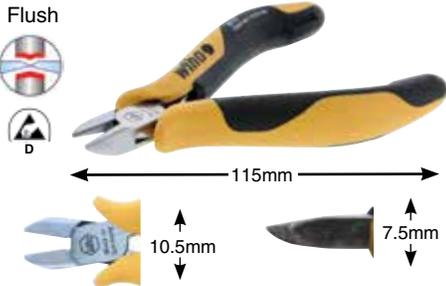
**32712 Precision Cutters, Slim Oval Head, Flush** Cutters drop-forged for an ideal material structure. Precise aligned cutting edges are additionally induction hardened at a hardness of Approx. 64°HRC. Two component non-slip soft grip handle, ESD Safe Dissipative.
