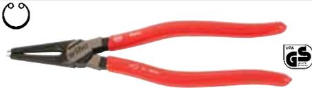
**326 Straight Internal Retaining Ring Pliers** DIN ISO 5256 Shape C, straight tips. Die forged cylindrical precision formed. Chrome-vanadium special tool steel. For inserting & removing internal retaining rings.
