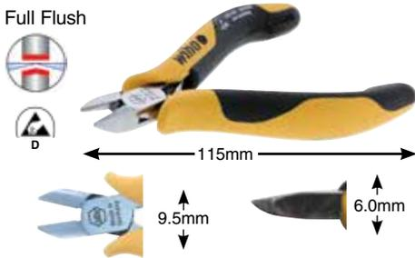
**32714 Precision Cutters, Slim Oval Head, Full Flush** Cutters drop-forged for an ideal material structure. Precise aligned cutting edges are additionally induction hardened at a hardness of Approx. 64°HRC. Two component non-slip soft grip handle, ESD Safe Dissipative.
