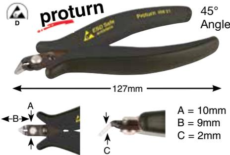
**45821 Protturn ESD Safe 45° Precision Cutters/Flush Cut** ESD standard IEC 61340-5-1. C70 special tool steel. Glare free, black finish. ESD Safe handle with non-slip grips.
