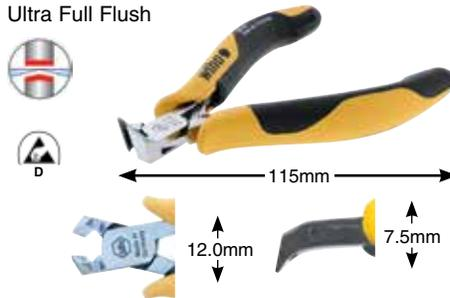
**32724 Oblique Angled Cutters, 29°, Full Flush** Oblique Cutters drop-forged for an ideal material structure. Precise aligned cutting edges are additionally induction hardened at a hardness of Approx. 64°HRC. Two component non-slip soft grip handle, ESD Safe Dissipative.
