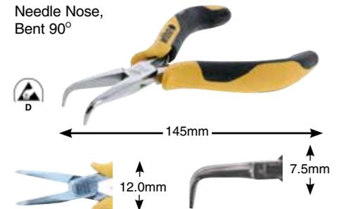
**32748 ESD Safe Pliers, Needle Nose Pliers, Bent 90°, Smooth Jaws** Pliers drop-forged for an ideal material structure. Precisely aligned, jaws, hardened. Two component non-slip soft grip handle, ESD Safe Dissipative.
