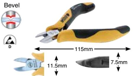
**32716 Precision Cutters, Wide Oval Head, Bevel** Cutters drop-forged for an ideal material structure. Precise aligned cutting edges are additionally induction hardened at a hardness of Approx. 64°HRC. Two component non-slip soft grip handle, ESD Safe Dissipative.
