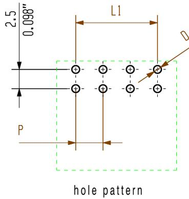
For the mounting of PCBs, it should be noted that the data given in the catalogue relates to the connection elements. The necessary creep clearance paths must be observed in connection with the respective applicant in accordance with VDE 0113. The current-carrying capacity and pitch tolerance must be determined according to DIN IEC 326 part 1.
