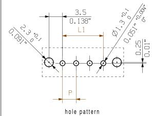
For the mounting of PCBs, it should be noted that the rated data given in the catalogue relates only to the connection elements. The neccessary creepage and clearance paths must be observed in connection with the respective applicant in accordance to VDE 0110. The current-carrying capacity and pitch tolerance is to be determined according to DIN IEC 326 part 3 very fine
