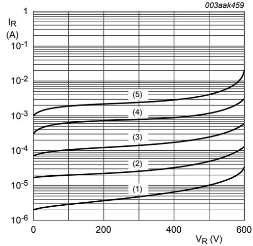
**Fig. 5. Reverse leakage current as a function of reverse voltage; typical values**
