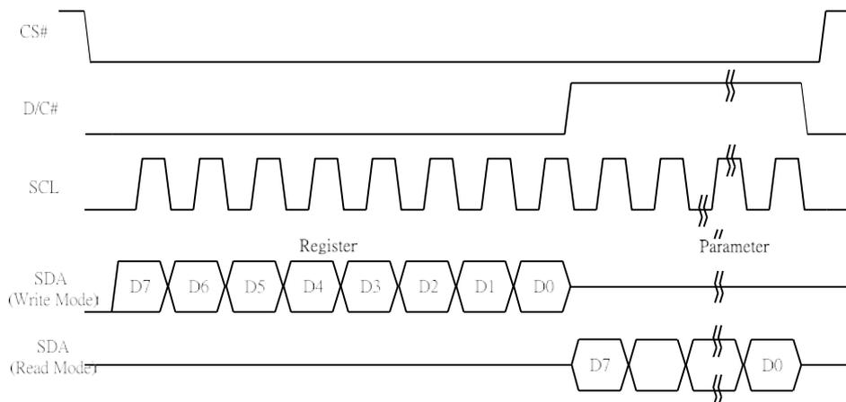
**Figure v-2: Read procedure in 4-wire SPI mode**
