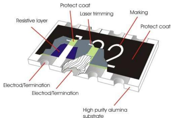
Fig 2. Construction of a Chip-R array (concave Type)
