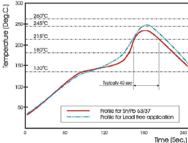
Fig 4. Infrared soldering profile for Chip Resistors array
