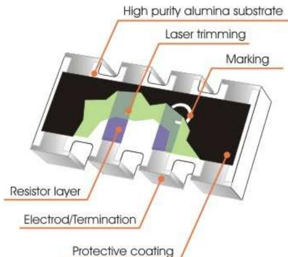
Fig 1. Construction of a Chip-R array (convex Type)
