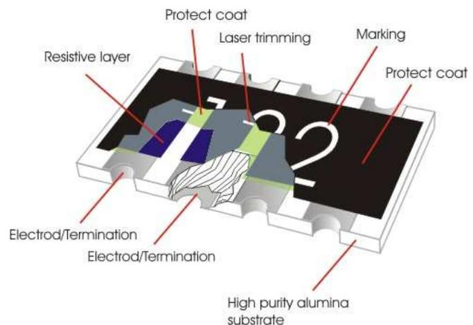
Fig 2. Construction of a Chip-R array (concave Type)
