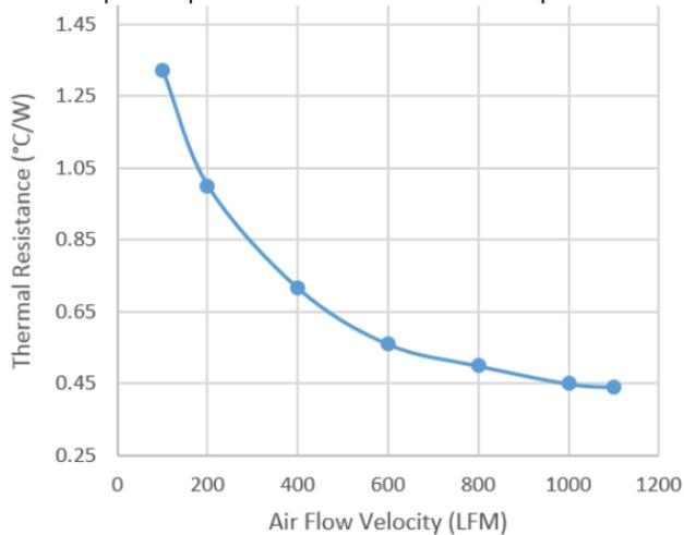
NOTE: Natural Convection Thermal resistance 2.10 °C/W based on 70 °C Temp rise about ambient.
