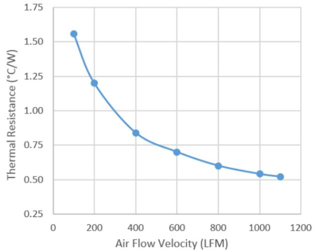
NOTE: Natural Convection Thermal resistance 2.50 °C/W based on 70 °C Temp rise about ambient.
