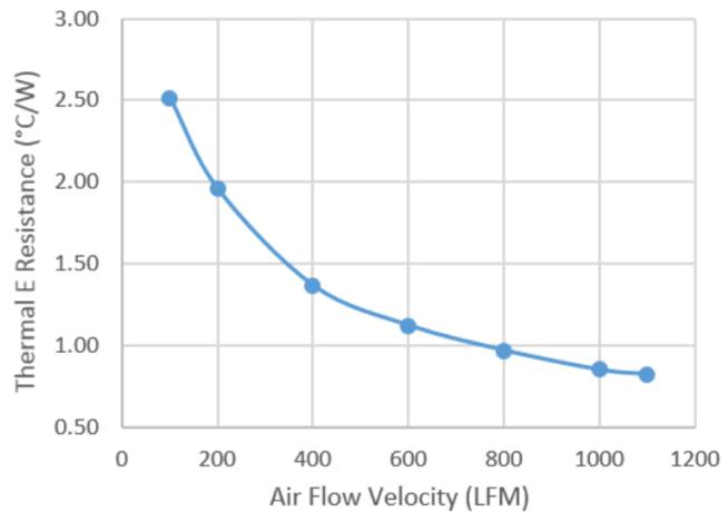
NOTE: Natural Convection Thermal resistance 4.06 °C/W based on 70 °C Temp rise about ambient.
