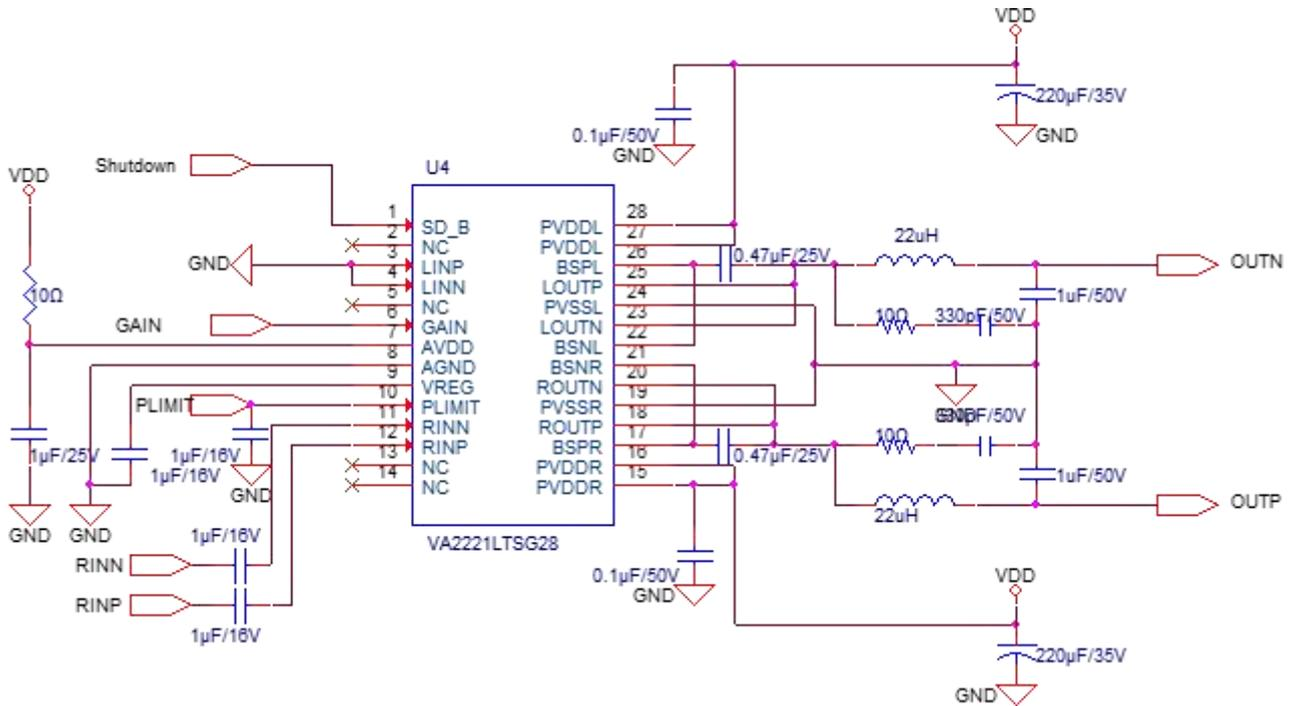
Figure 7. VA2221L Mono Reference Application with LC Filter
