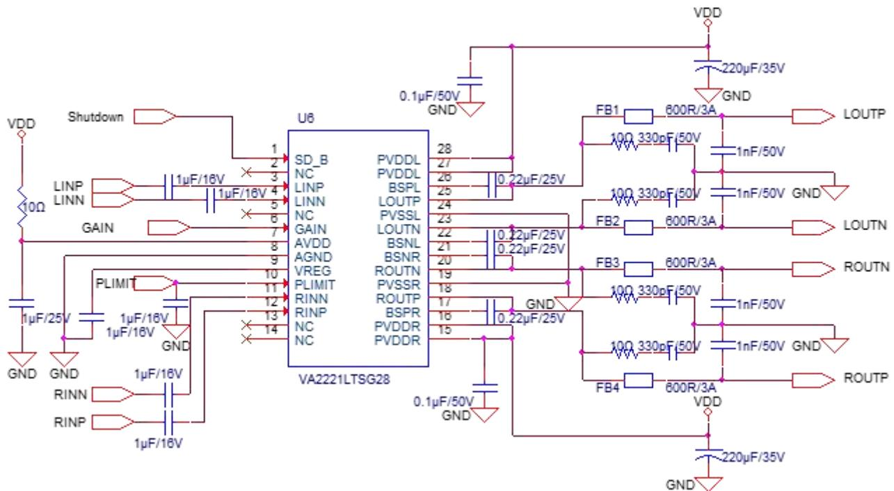
Figure 6. VA2221L Stereo Reference Application with Ferrite Bead
