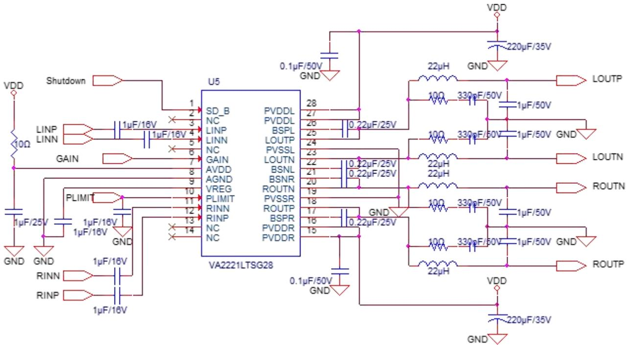
Figure 5. VA2221L Stereo Reference Application with LC Filter
