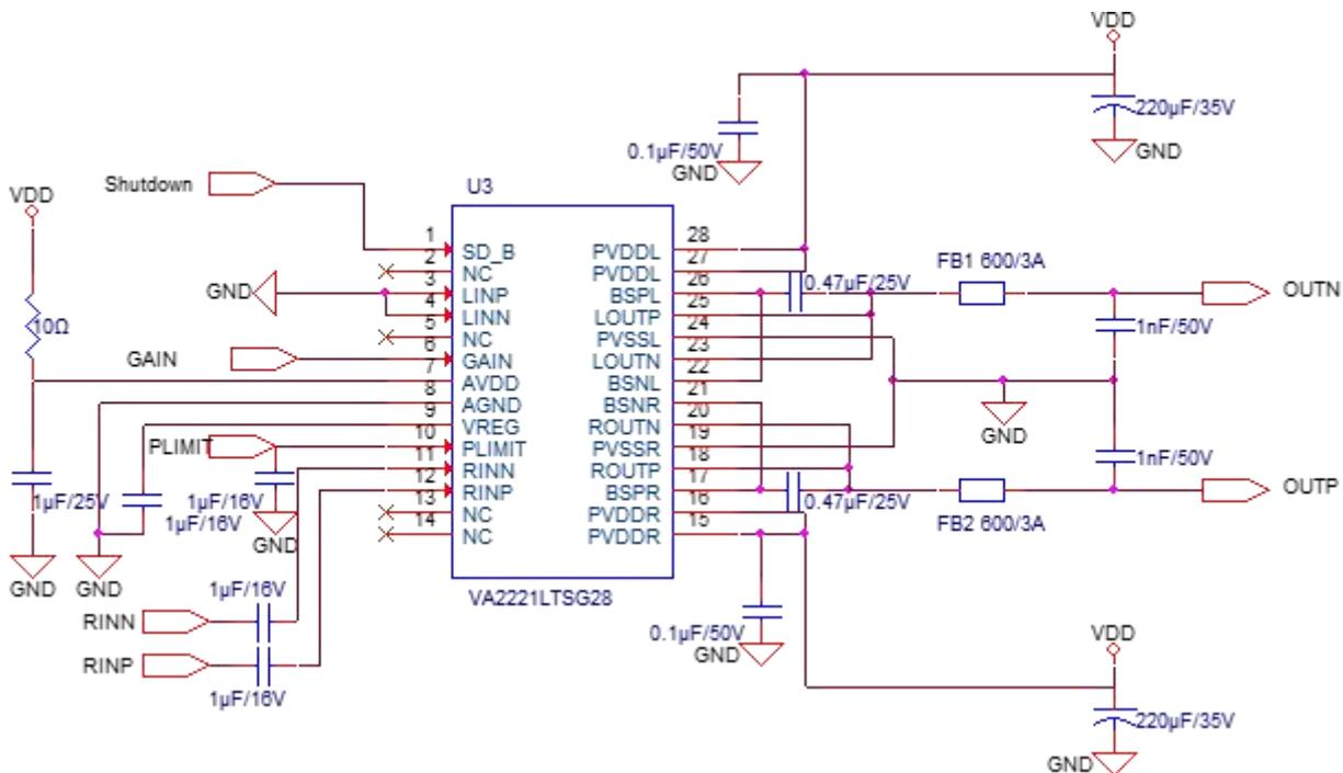
Figure 8. VA2221L Mono Reference Application with Ferrite Bead
