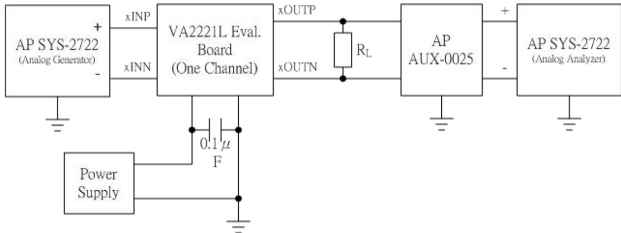
\* Remove all L/C (BEAD) filter components on board before performing all measurements.
