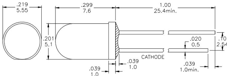
\* Tolerance :  $\pm \frac{0.01}{0.25}$  Unit :  $\pm \frac{\text{inch}}{\text{mm}}$
