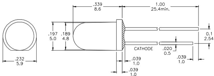
\* Tolerance :  $\pm \frac{0.01}{0.25}$  Unit :  $\pm \frac{\text{inch}}{\text{mm}}$
