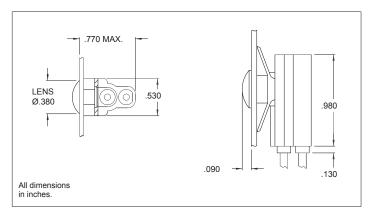
Mounting: Will snap-fit into Ø.032/.317 in panels .202/.125 thick.
