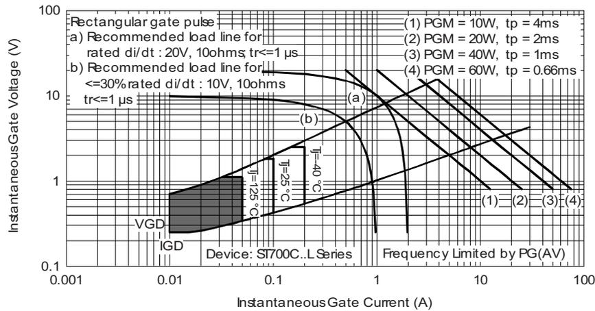
Fig. 11 - Gate Characteristics
